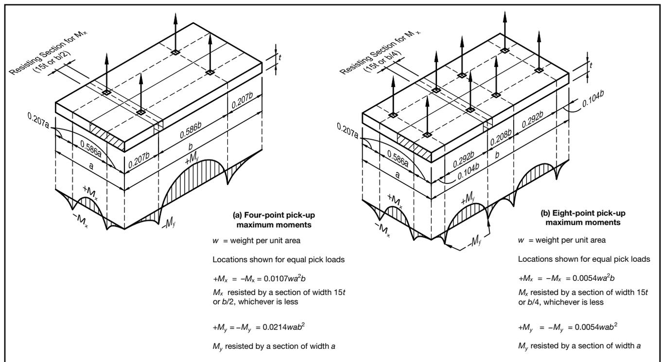
Moments developed in panels stripped flat. Source: Figure 8.3.2 from the eighth edition *PCI Design Handbook: Precast and Prestressed Concrete*.
