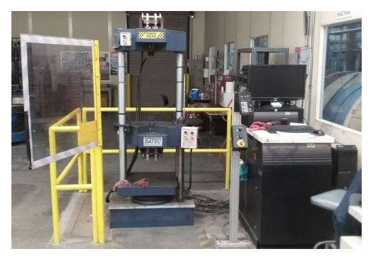
Figure 1 – Example of test frame and data acquisition system used for tensile testing of strands
