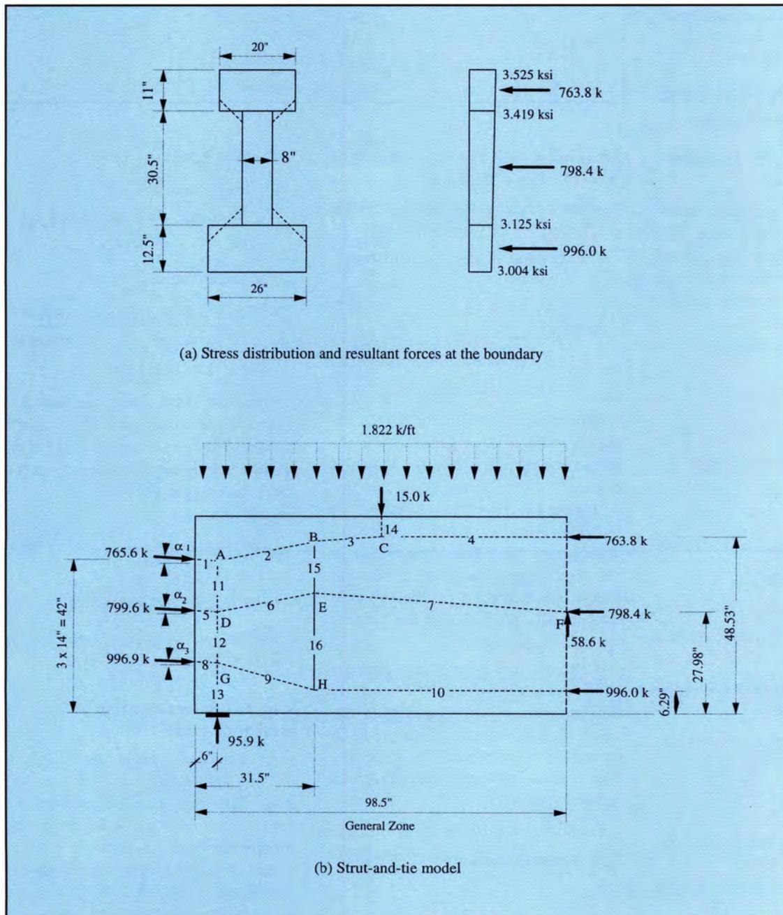
Fig. B2. Strut-and-tie model. (a) Stress distribution and resultant forces at boundary; (b) Strut-and-tie model.
