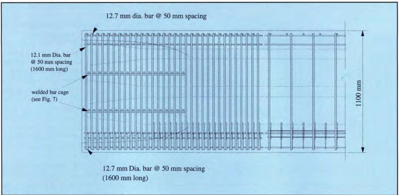
Fig. 8. Reinforcement details (Detail 2).
