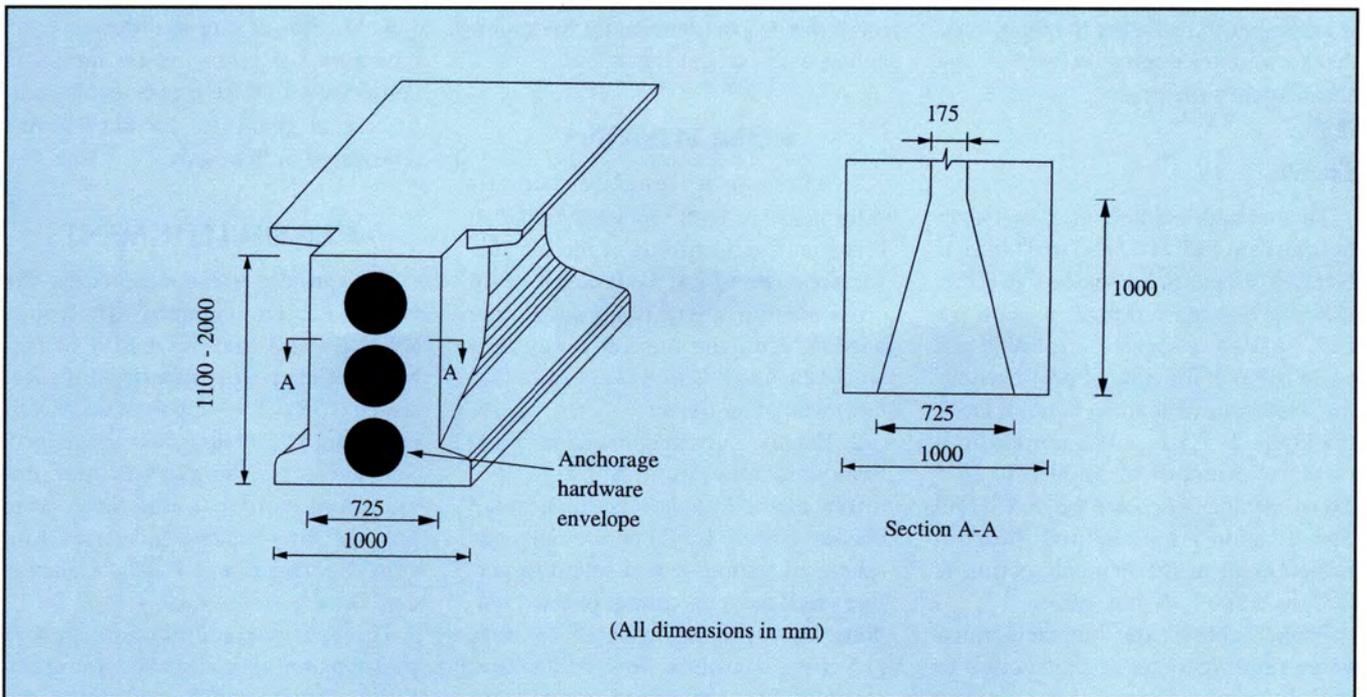
Fig. 16. Standard NU I-beam post-tensioning anchorage (concrete dimension).
