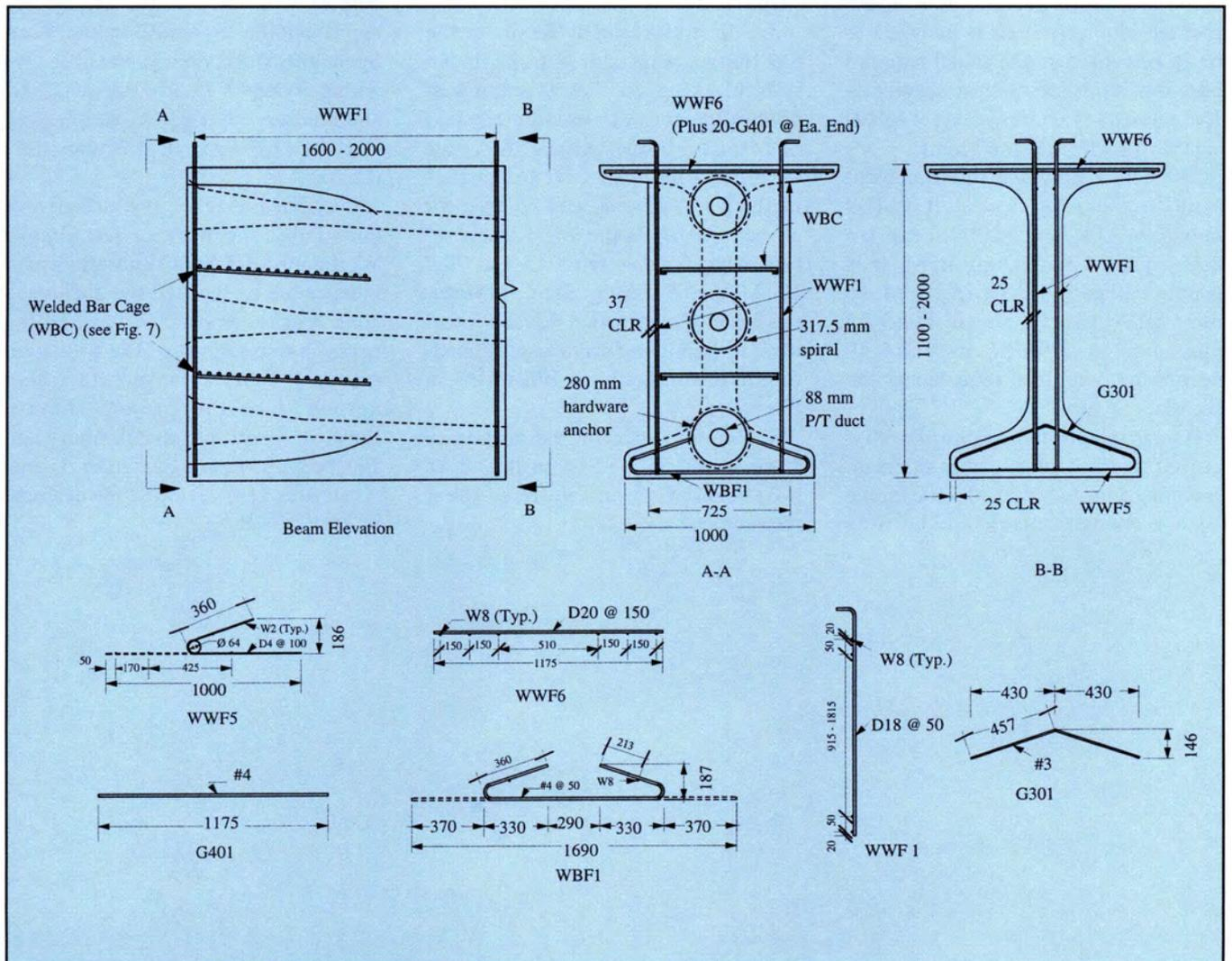
Fig. 17. Standard NU I-beam post-tensioning anchorage (reinforcement).
