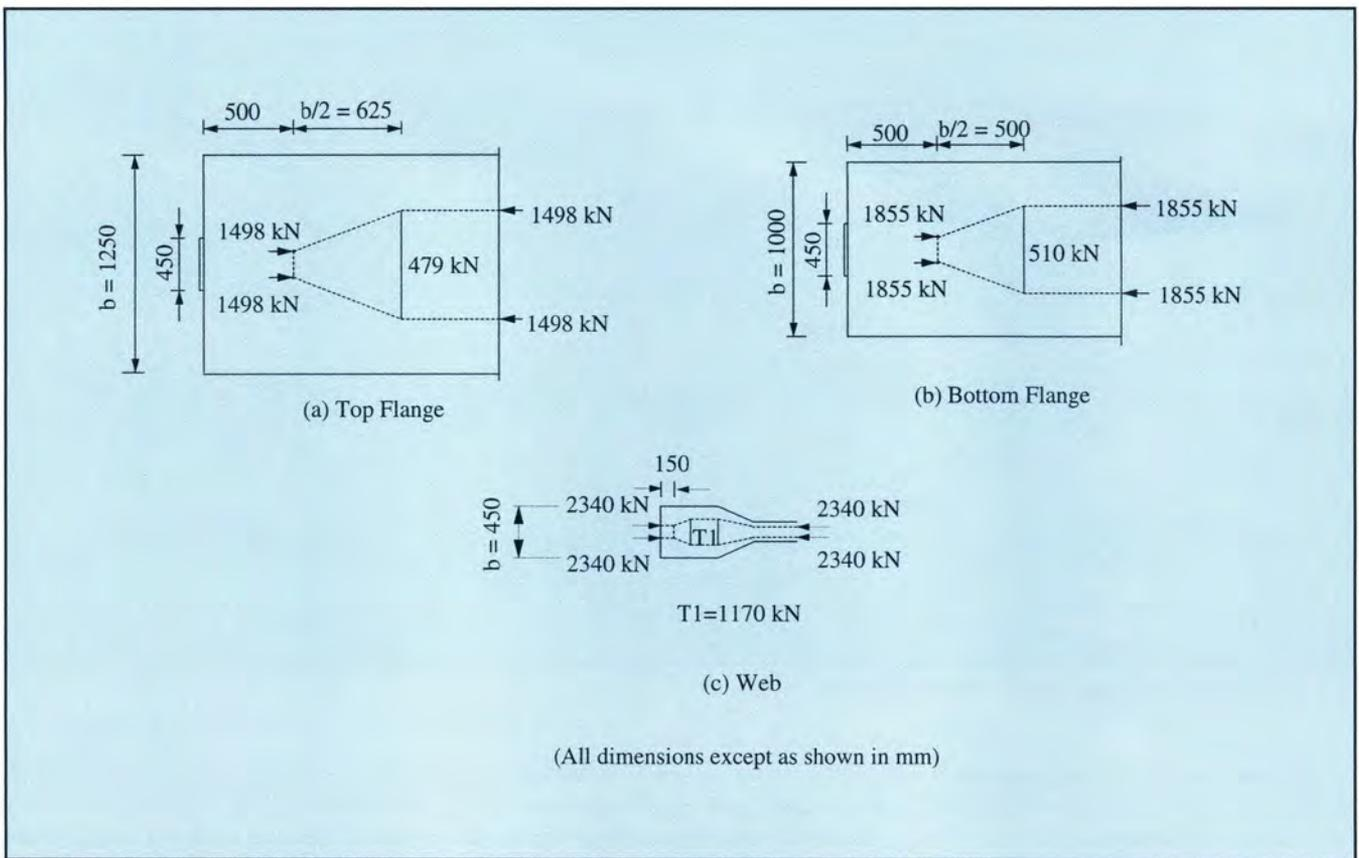
Fig. 4. Strut-and-tie models in transverse direction (Detail 1).
