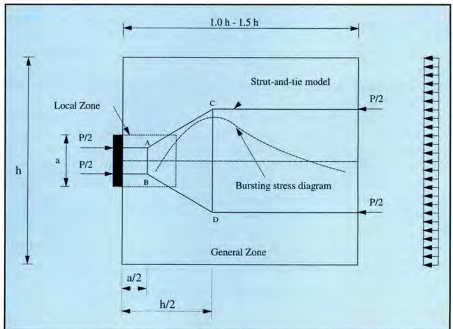
Fig. 1. Force flow of a simple anchorage zone.
