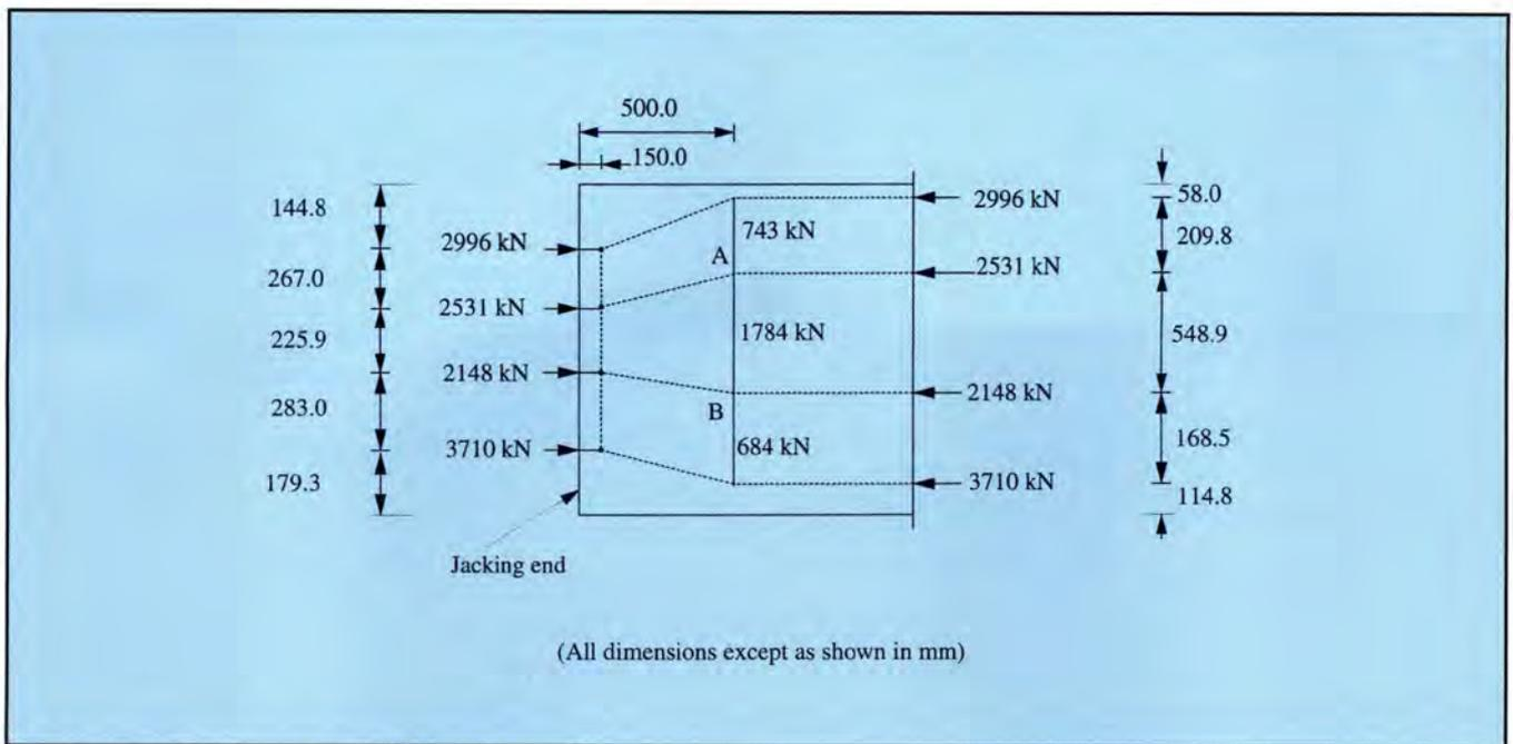
Fig. 3. Strut-and-tie model in beam height direction.
