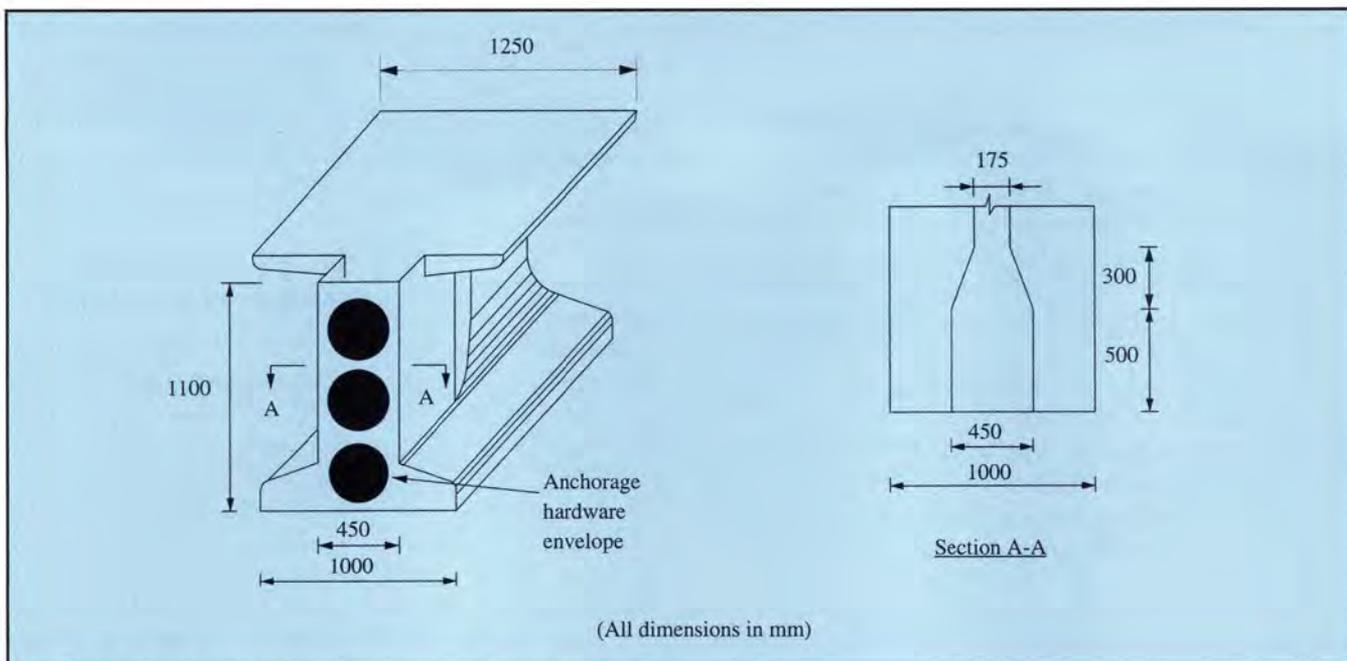
Fig. 2. Detail 1 — Optimized rectangular anchorage zone.
