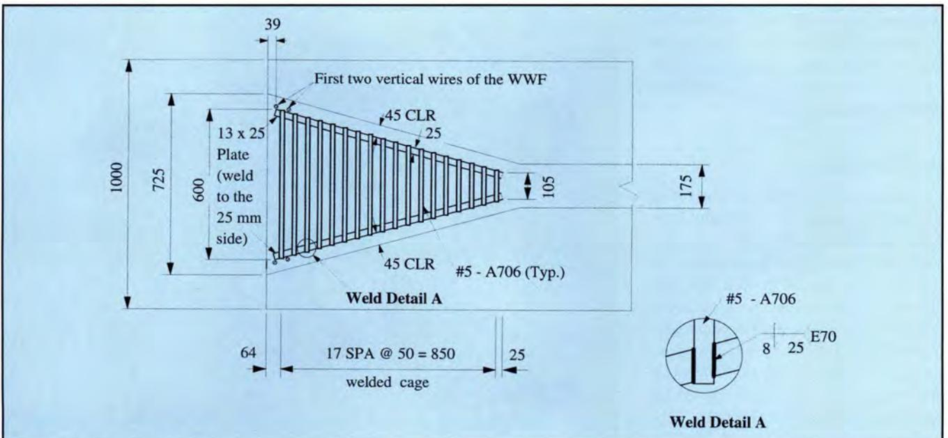
Fig. 7. Welded bar cage detail.
