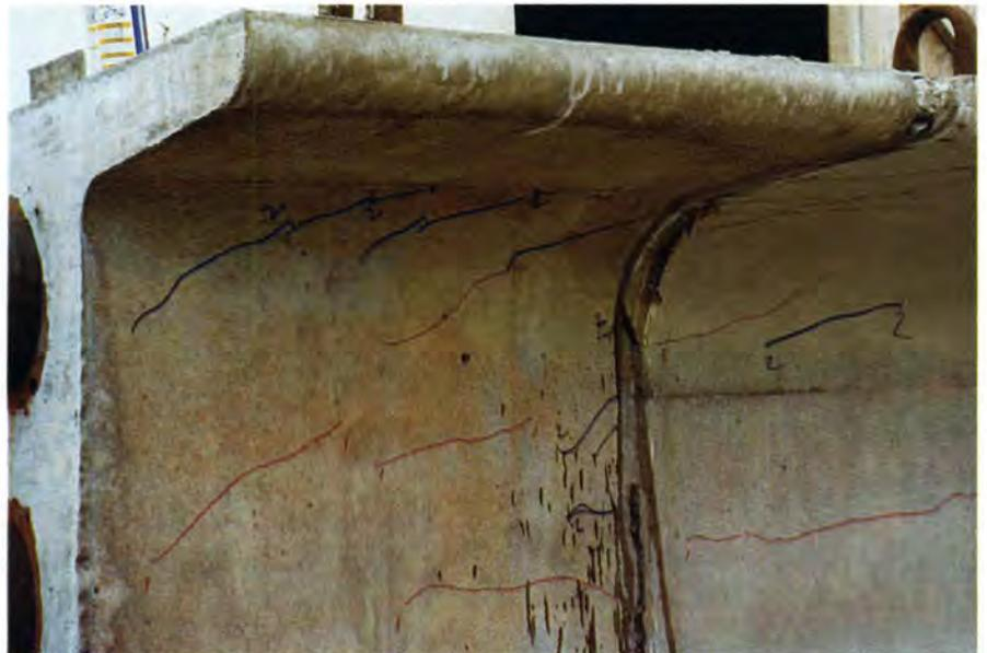
Fig. 11. Hairline cracks after post-tensioning (Detail 1).
