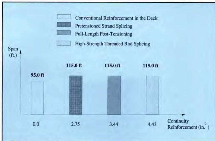
Fig. 8. Span capacity of NU 1100 I-beam.
