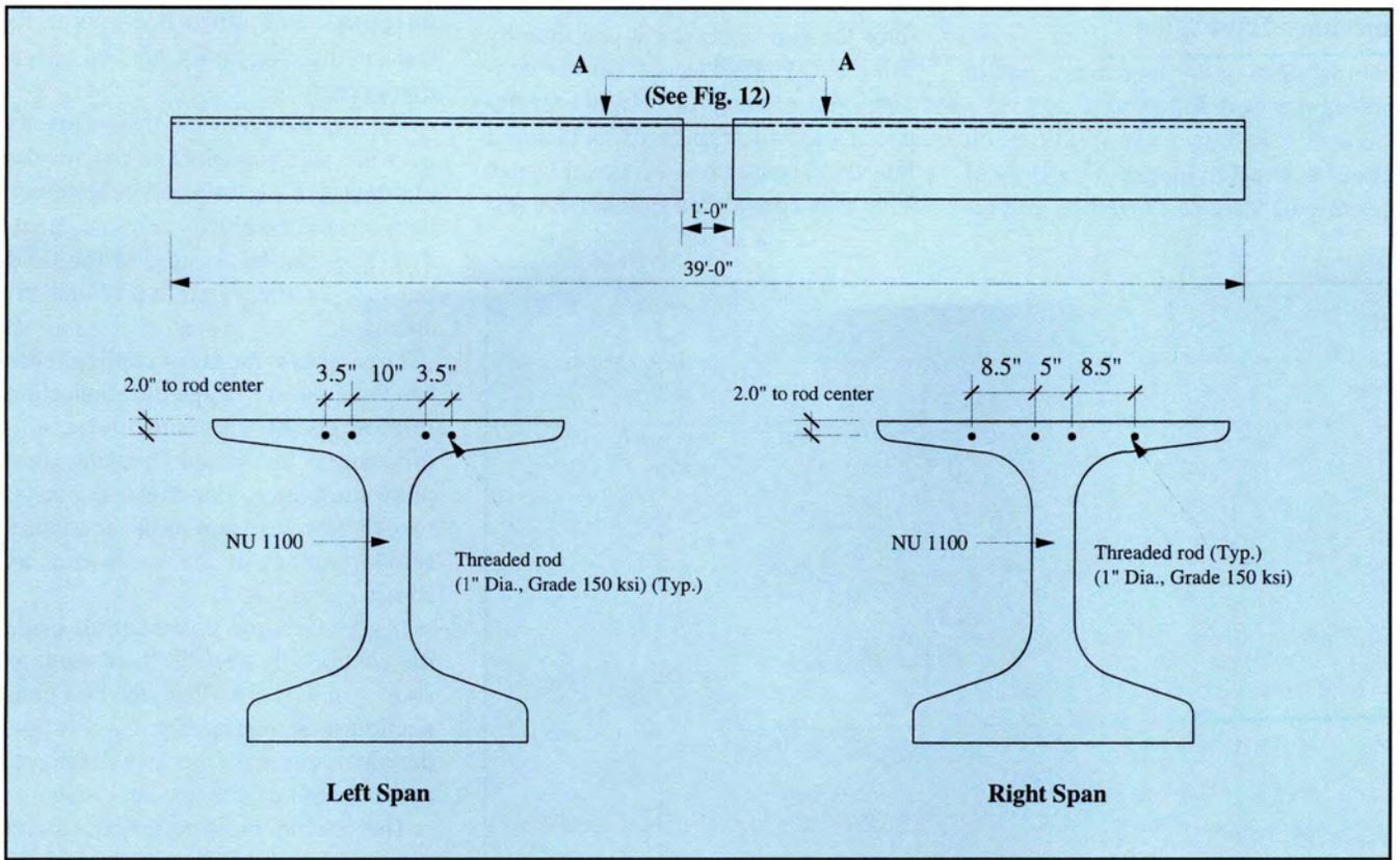
Fig. 11. Continuity for deck weight by Grade 150 ksi (1034 MPa) threaded rods (Specimen CB).
