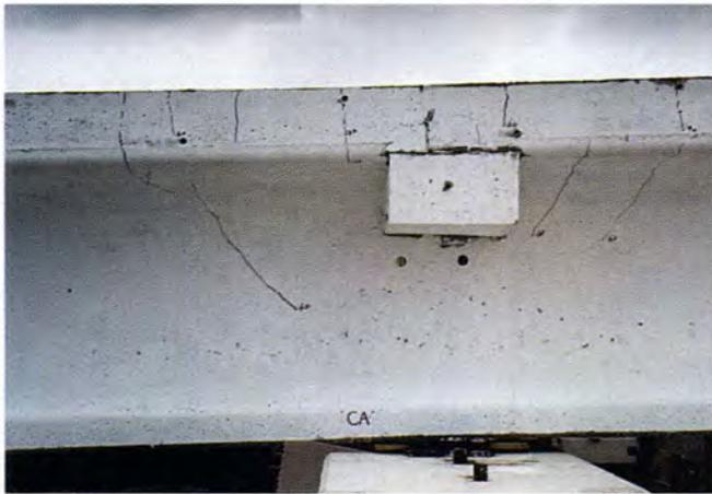
Fig. 22. First stage of cracks of Specimen CA.
