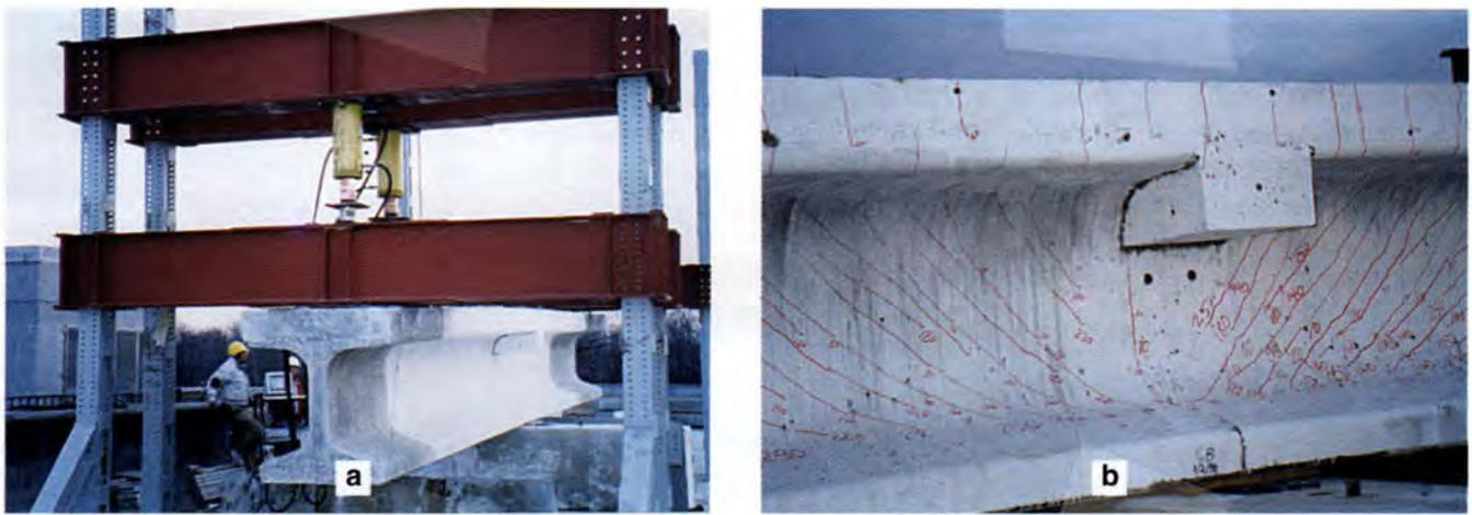
Fig. 25. Maximum loading stage of Specimen CB. (a) Large deflection (b) Closely spaced cracks
