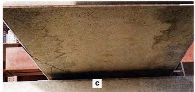
Fig. 24. Unsymmetrical failure of Specimen CA.
