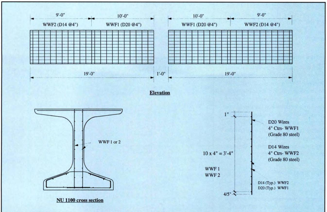
Fig. 15. Orthogonal WWR shear reinforcement (Specimens CA, CB, and CC).
