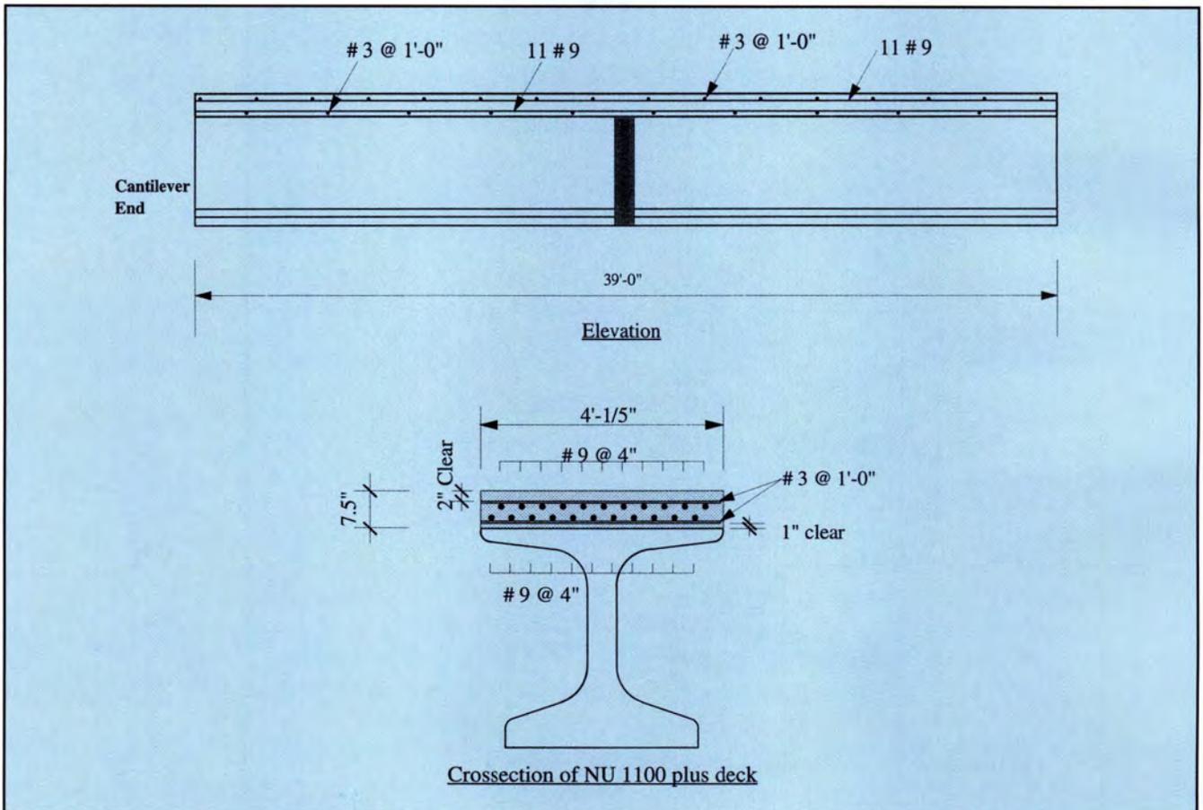
Fig. 14. Continuity reinforcement in deck for superimposed dead and live load (Specimens CA, CB, and CC).
