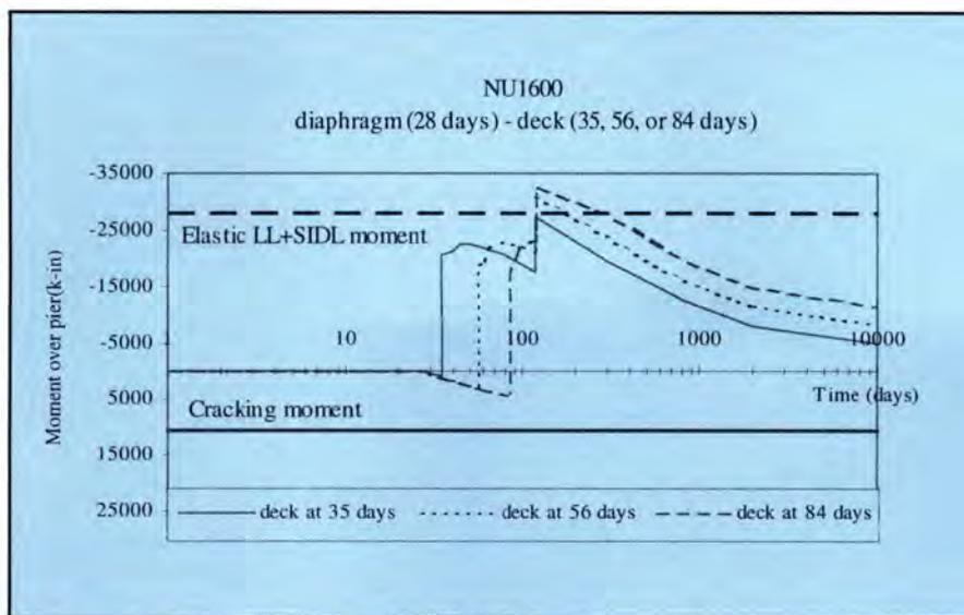
Fig. 7. Time-dependent moment due to diaphragm and deck separate casting.
