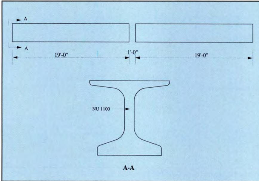
Fig. 13. No continuity reinforcement in beam for Specimen CC.
