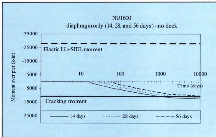
Fig. 4. Time-dependent moment due to diaphragm only (NU1600).
