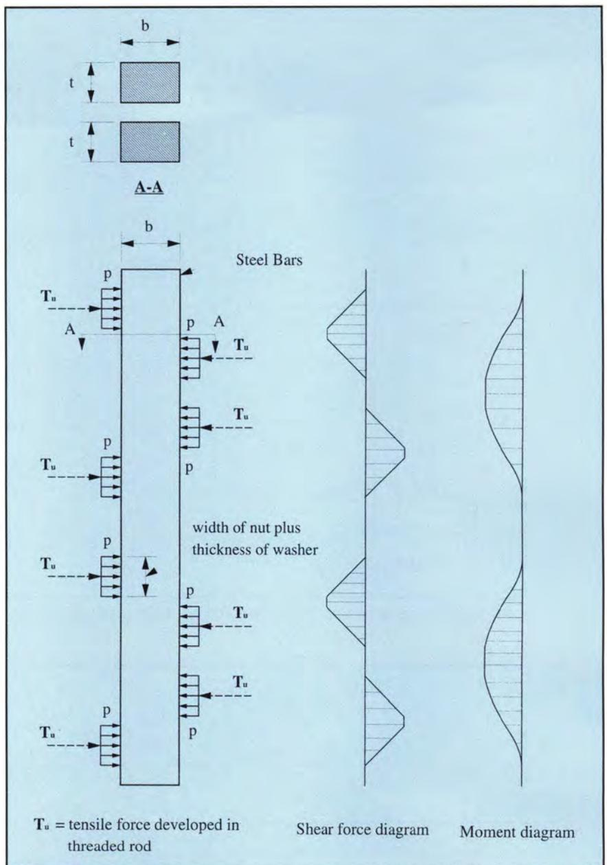
Fig. 17. Design of rectangular steel bars.
