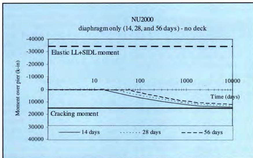
Fig. 5. Time-dependent moment due to diaphragm only (NU2000).
