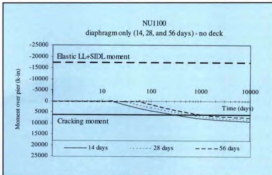
Fig. 3. Time-dependent moment due to diaphragm only (NU1100).
