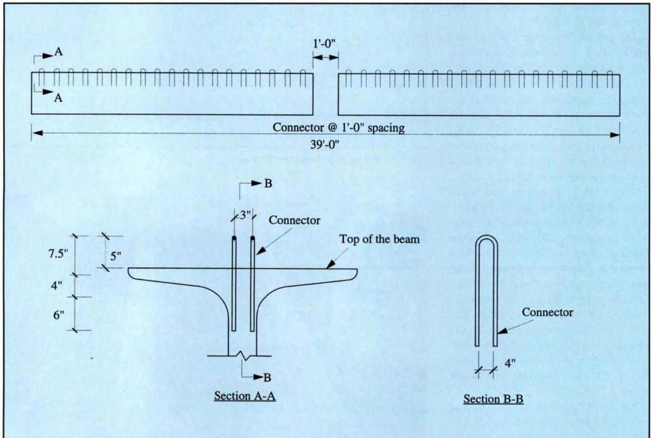
Fig. 16. Connector details (Specimens CA, CB, and CC).
