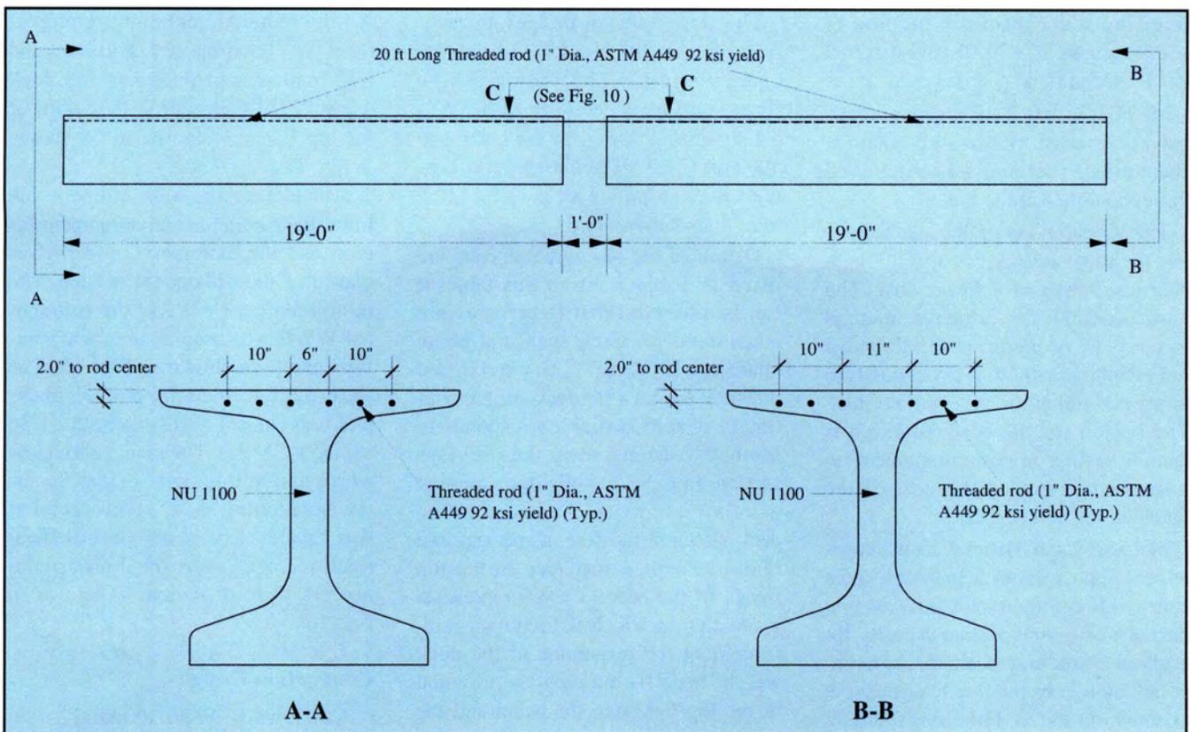
Fig. 9. Continuity for deck weight by Grade 92 ksi (634 MPa) threaded rods (Specimen CA).
