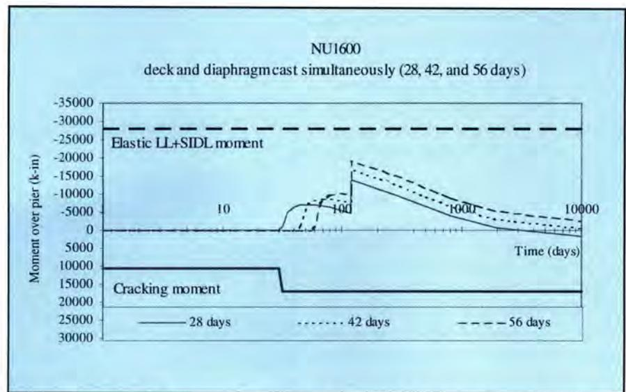
Fig. 6. Time-dependent moment due to diaphragm and deck simultaneous casting.
