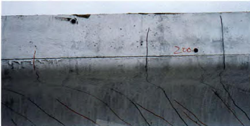
Fig. 26. Delamination of deck slab of Specimen CC.
