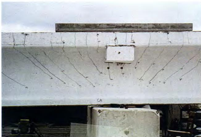
Fig. 23. Fan shape of flexural-shear cracking.
