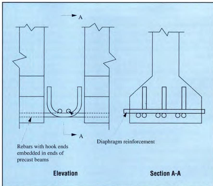
Fig. 1. Positive restraint moment connection details by embedded reinforcing bars.
