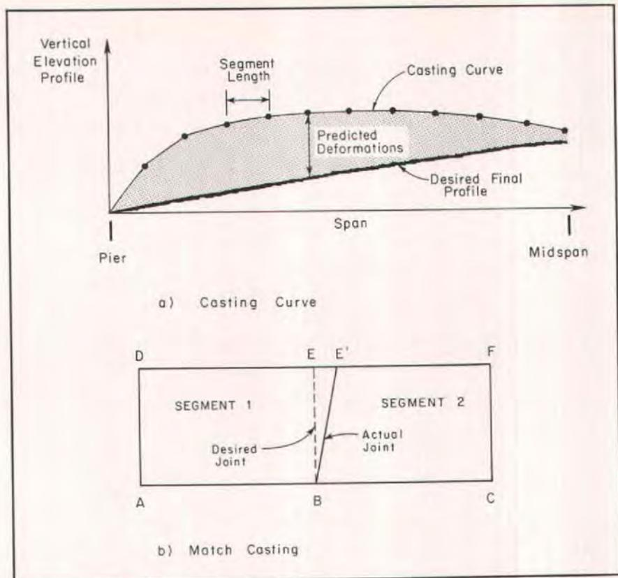
Fig. 4. Basis of match casting in segmental construction.
