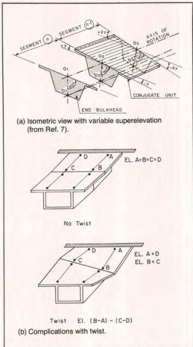
Fig. 11. Short line casting — Variable superelevation.
