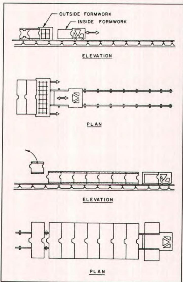
Fig. 5. Match casting systems (from Ref. 6).
