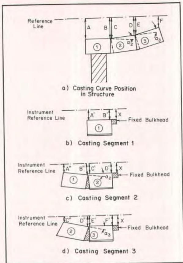
Fig. 7. Vertical elevation geometric control during casting operations.
