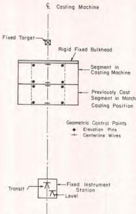
Fig. 6. Short line method geometric control.
