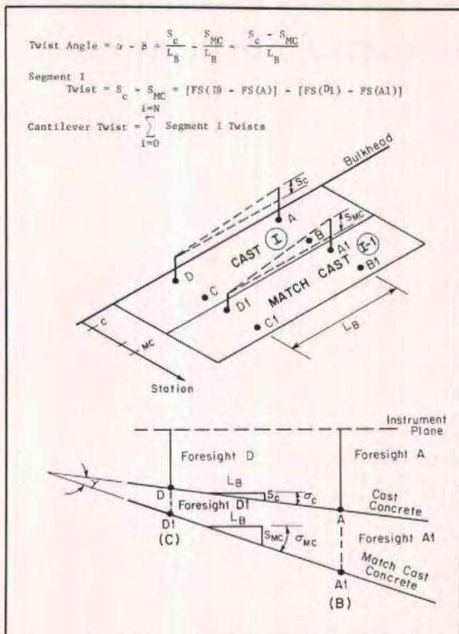
Fig. 12. Determination of segment twist directly from casting yard measurement.
