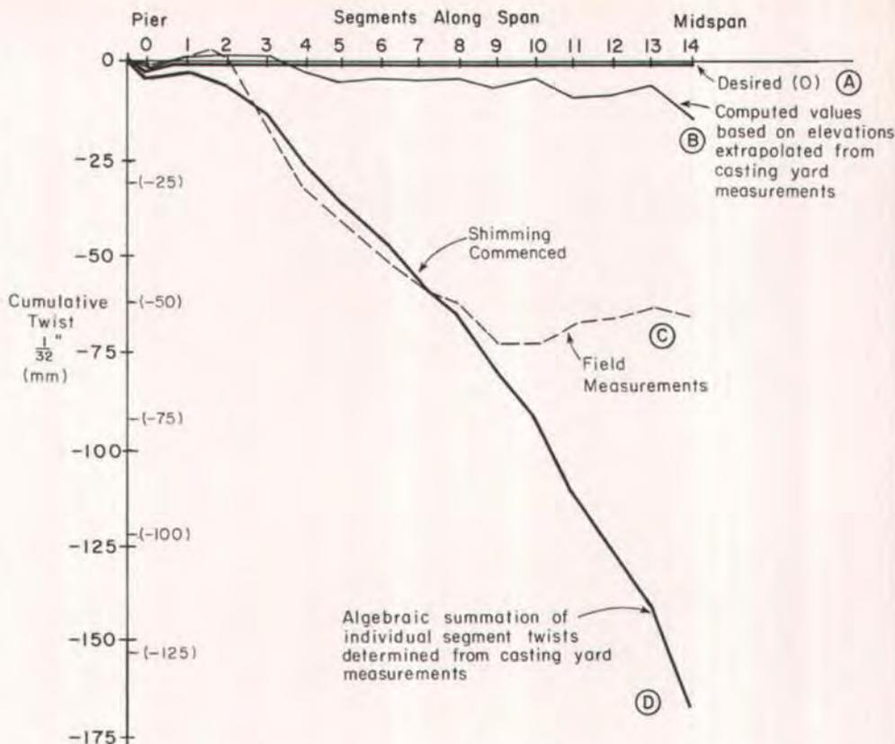
Fig. 18. Twist measurements with effective field shimming as a control measure.
