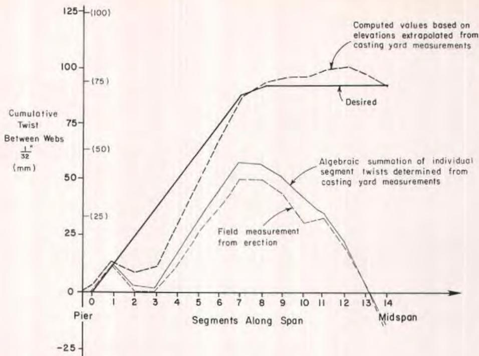
Fig. 17. Desired and measured cumulative twist values.
