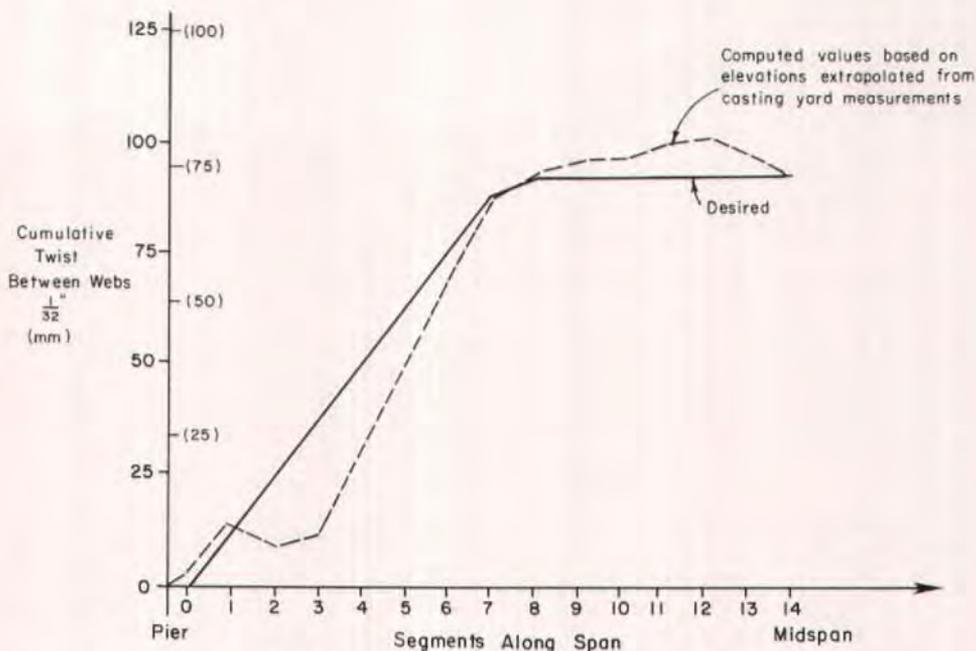
Fig. 15. Desired and computed cumulative twist values.
