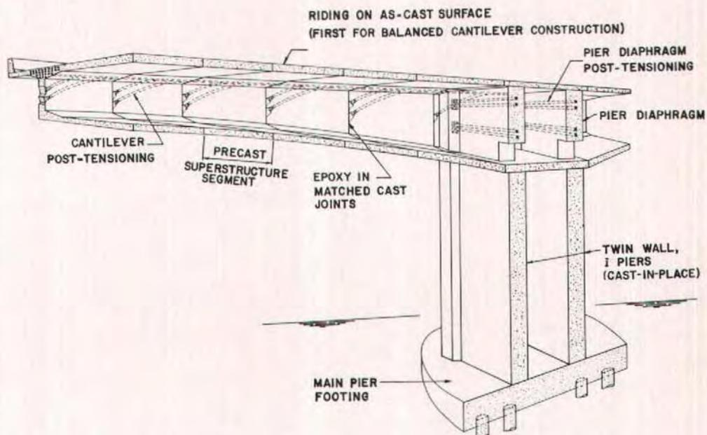
Fig. 5. Cutaway section of bridge at start of 400-ft (122 m) main span, showing major features of construction method.
