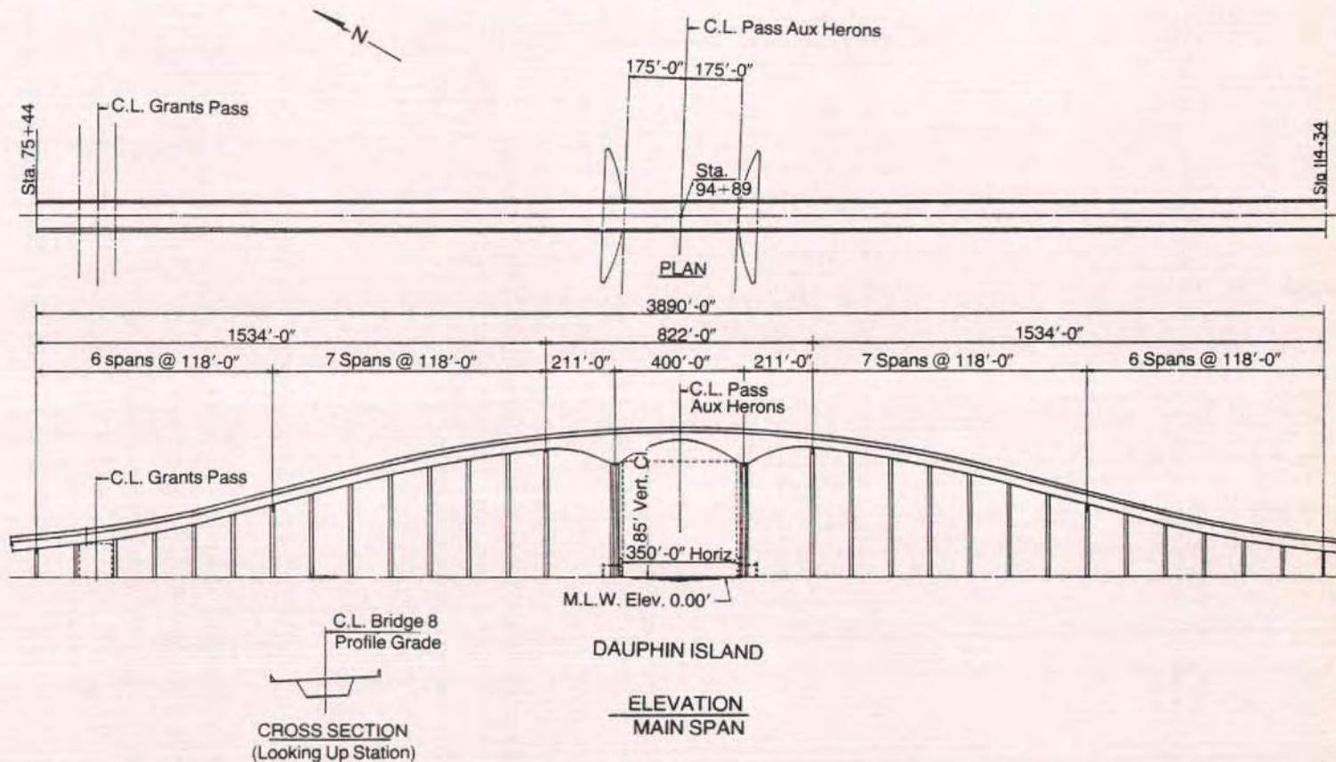
Fig. 7. Plan and elevation of main span of Dauphin Island Bridge. (Note: 1 ft = 0.305 m; 1 in. = 25.4 mm.)
