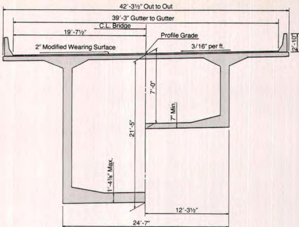
Fig. 8. Half section of variable depth box segments for 400-ft (122 m) main span of Dauphin Island Bridge. (Note: 1 ft = 0.305 m; 1 in. = 25.4 mm.)
