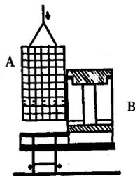
(b) Transfer bottom flange forms to A and place reinforcement for webs in half segment A
