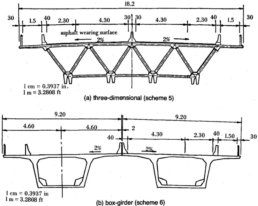
Fig. 7. Alternate superstructure cross sections.
