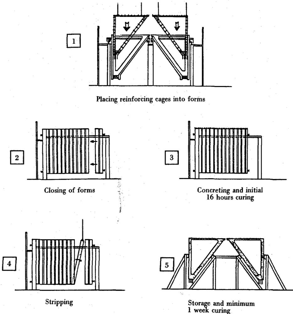
Fig. 18. Schematic of triangle fabrication.
