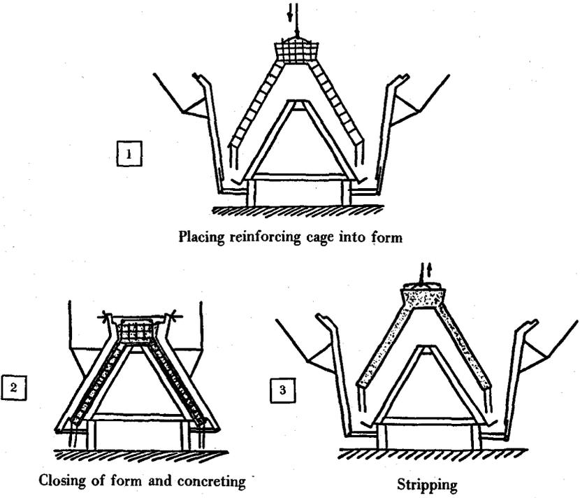
Fig. 19. Fabrication schematic of pier segment diagonals.
