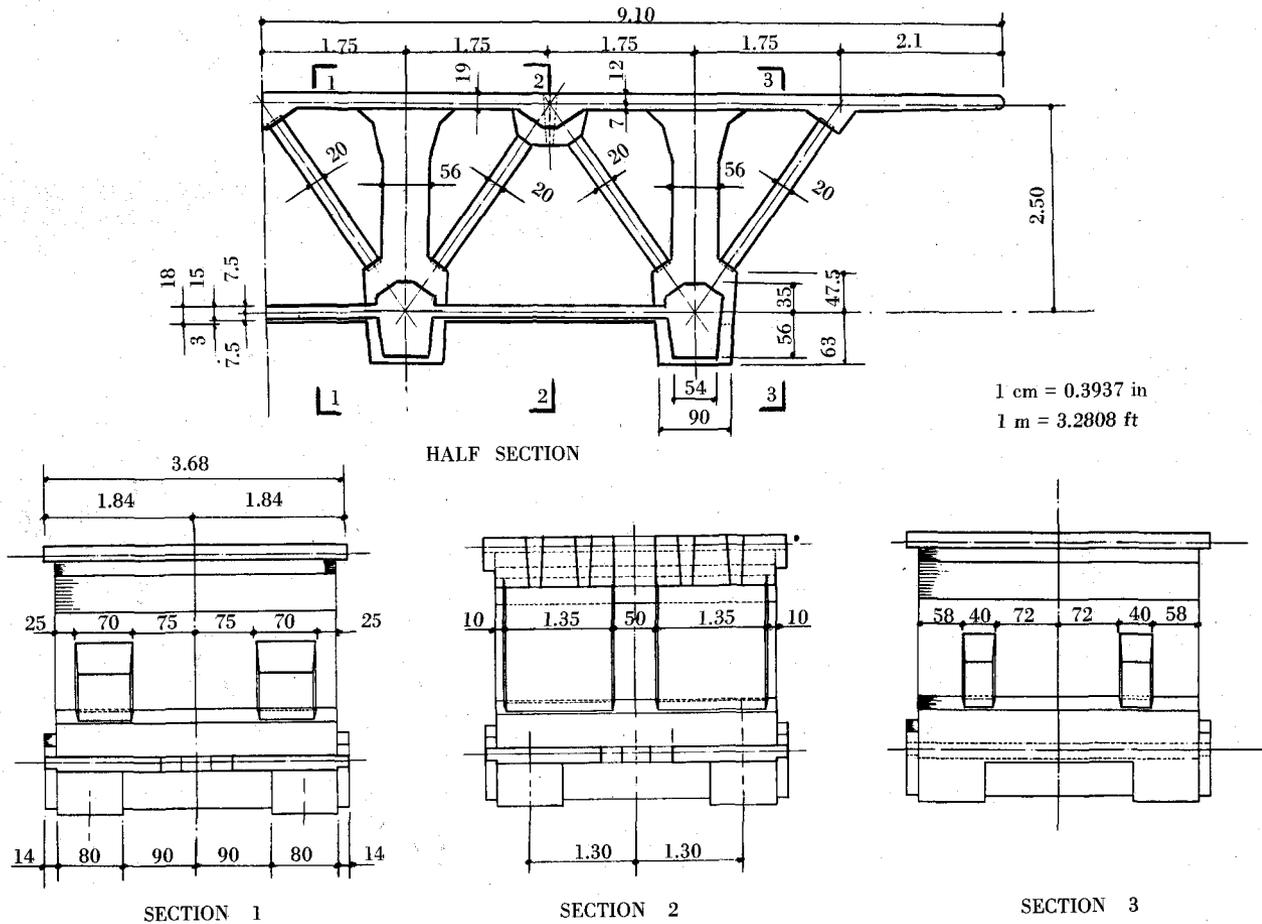
Fig. 12. Details of a pier segment showing various sections.
