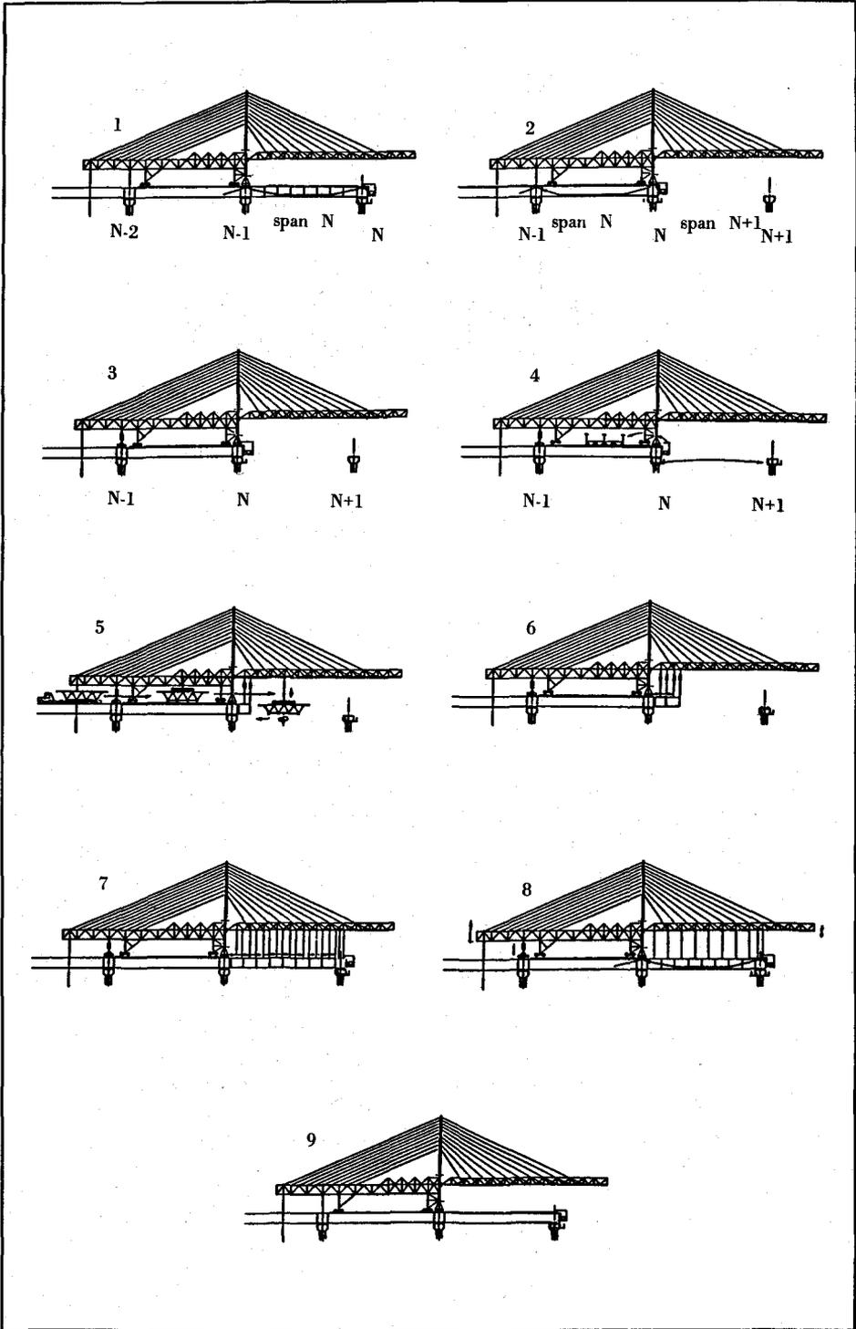
Fig. 27. Schematic erection sequence of a typical span.
