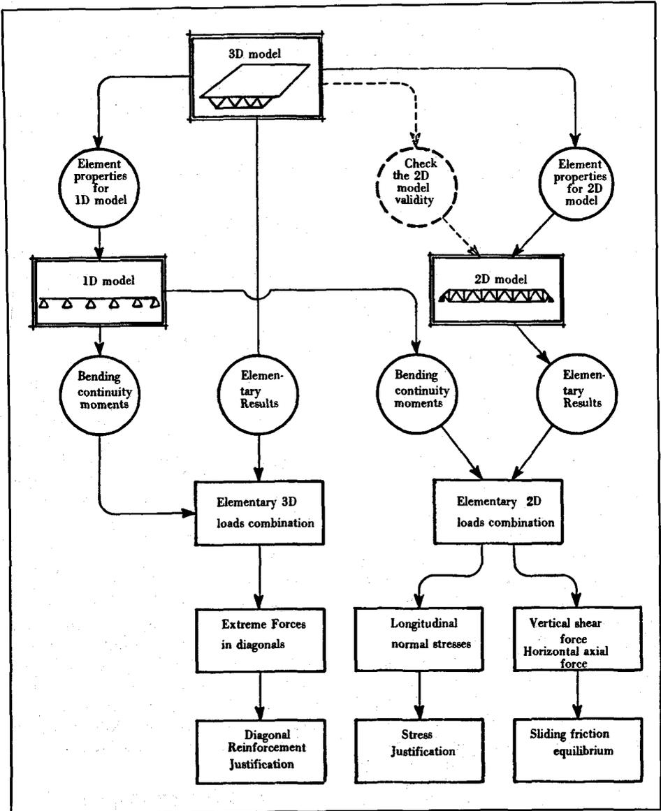
Fig. 14. Linking of FASTRUDL computer models.
