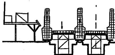
(c) Place bottom flange reinforcement in half segment A
