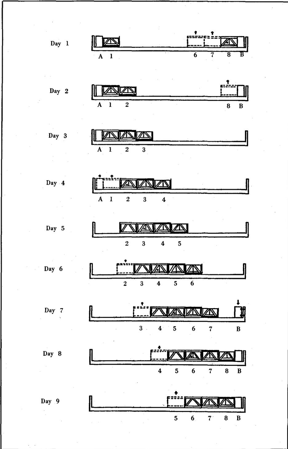
Fig. 26. Schematic casting cycle for typical segments.
