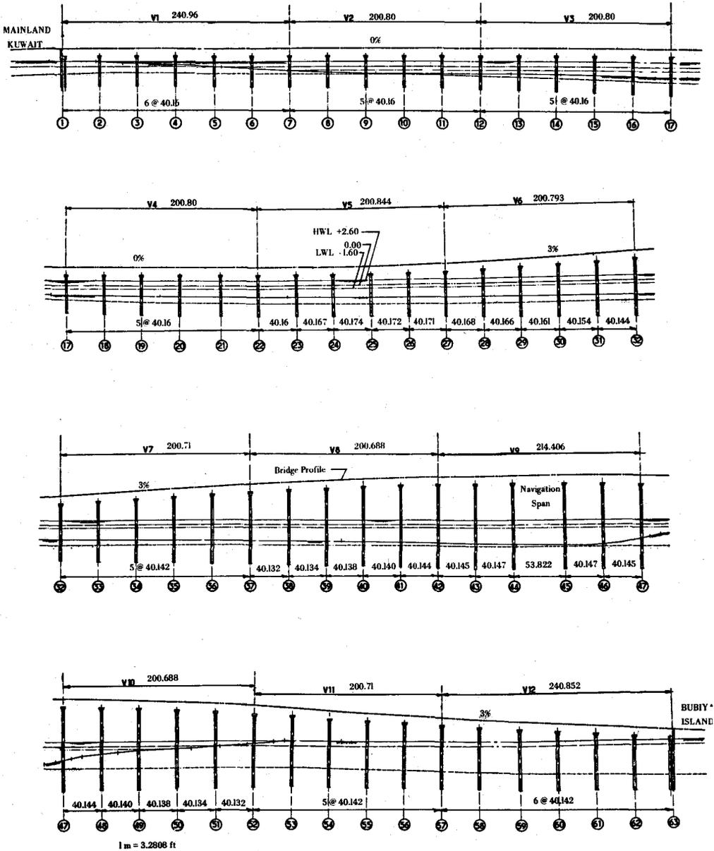
Fig. 6. Elevation of Bubiyan Bridge showing span arrangement. See Fig. 34 for final design modifications to structure for Bubiyan Island ramp.
