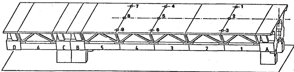
Fig. 33. Isometric of test model showing location of tensioning bars.
