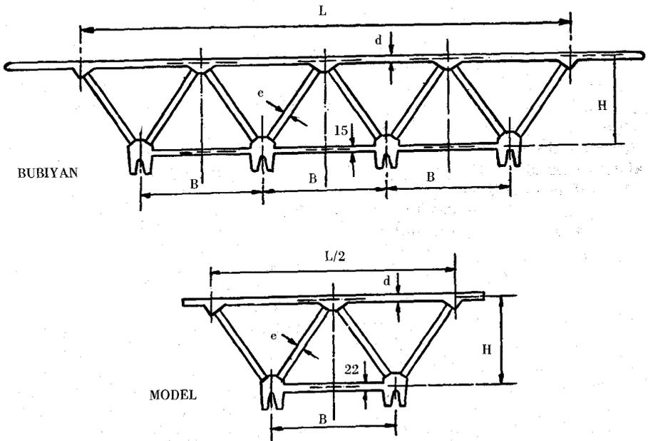
Fig. 32. Comparison of test model and Bubiyan Bridge cross section.
