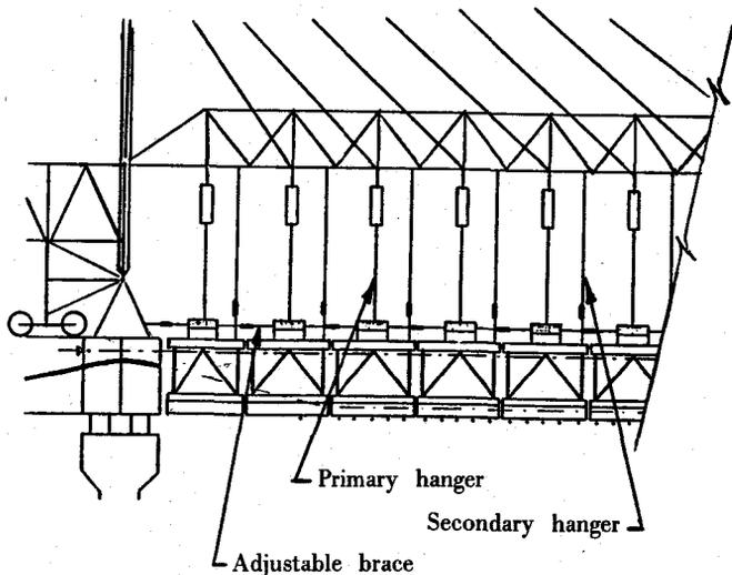
Fig. 28. Schematic of launching girder support hangers.
