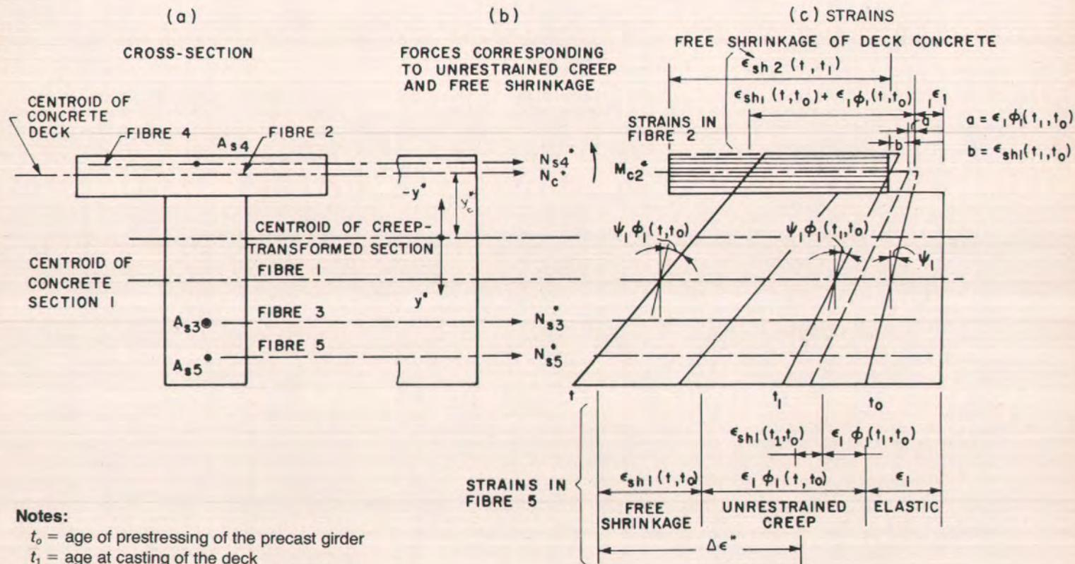
Fig. 6. Strains in composite girder due to initial forces on girder, unrestrained creep and free shrinkage.
