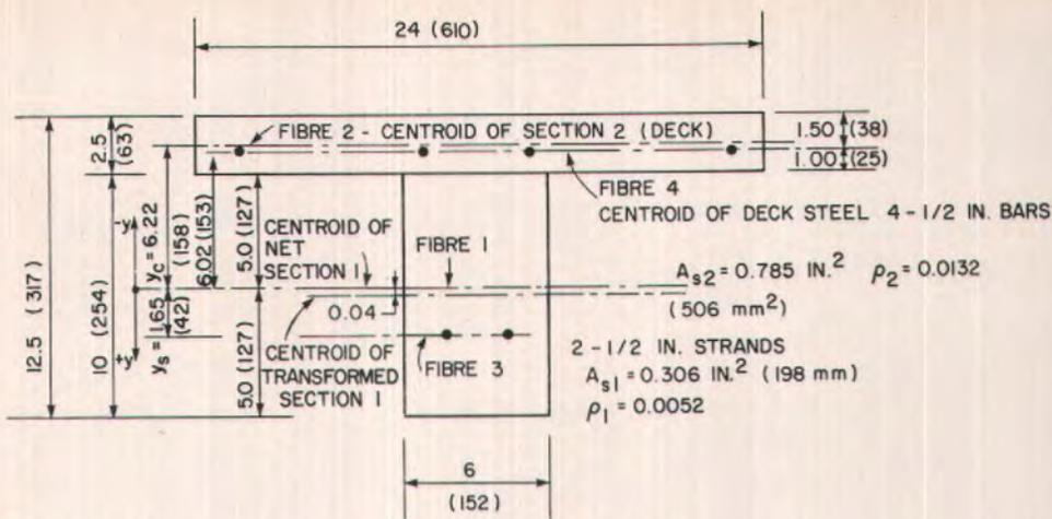
Fig. 7. Cross section of the composite girder of Example 2.
