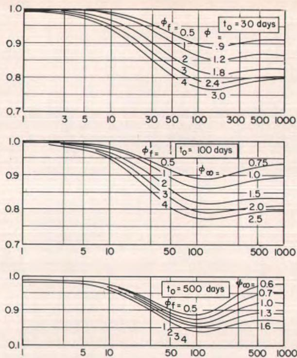
**Note:**  $\phi_f$  is the flow coefficient according to Reference 6;  $\phi_\infty$  is the ultimate creep coefficient  $\phi(t_\infty, t_0)$  determined with  $E_c(t_0)$ .
