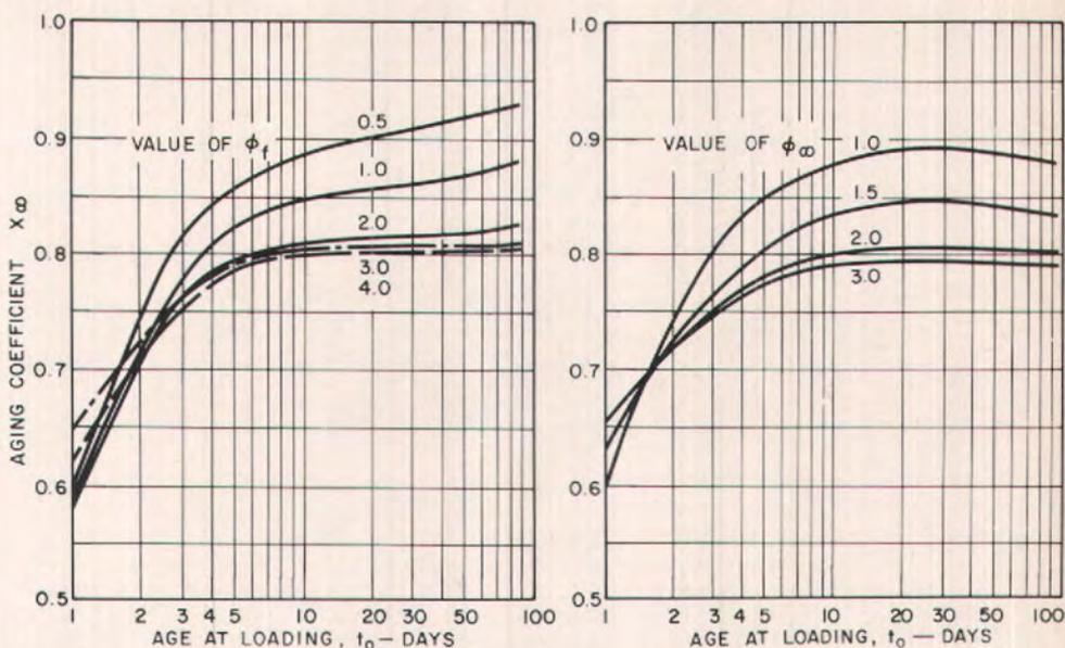
(a) For different values of the flow coefficient  $\phi_f$  (according to Reference 6).
