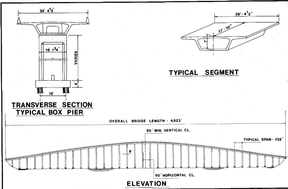
Fig. 5. Typical segment, pier section, and elevation of Channel No. 5 Bridge, Florida Keys. (Courtesy: Figg and Muller Engineers, Inc.)
