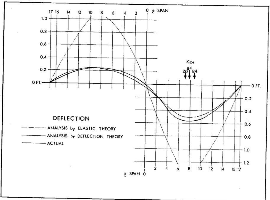
Fig. 17—94 Ton Test Load—Stiffening Girder Deflections
