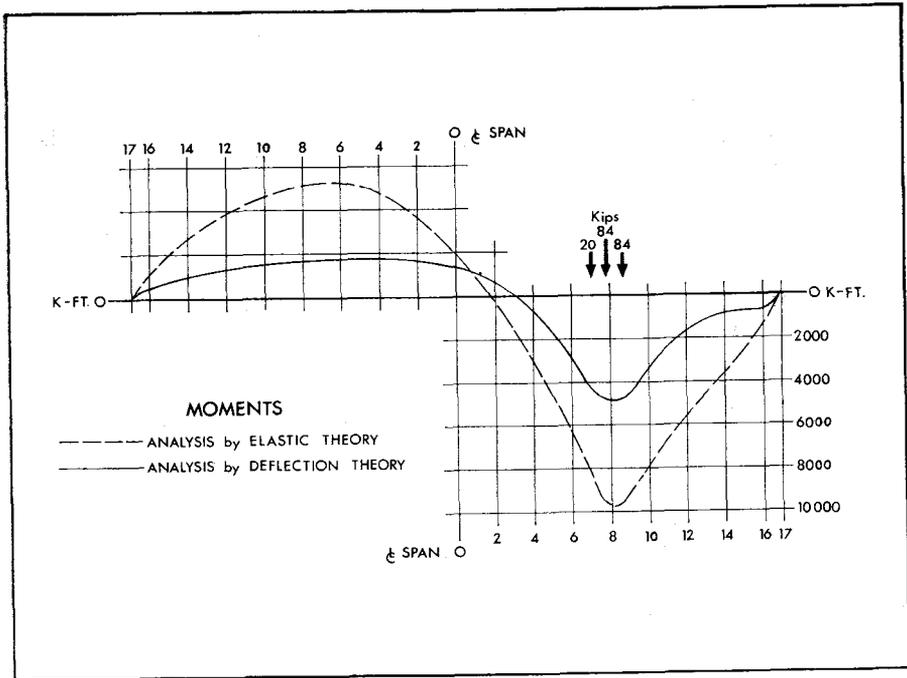
Fig. 18—94 Ton Test Load—Stiffening Girder Moments
