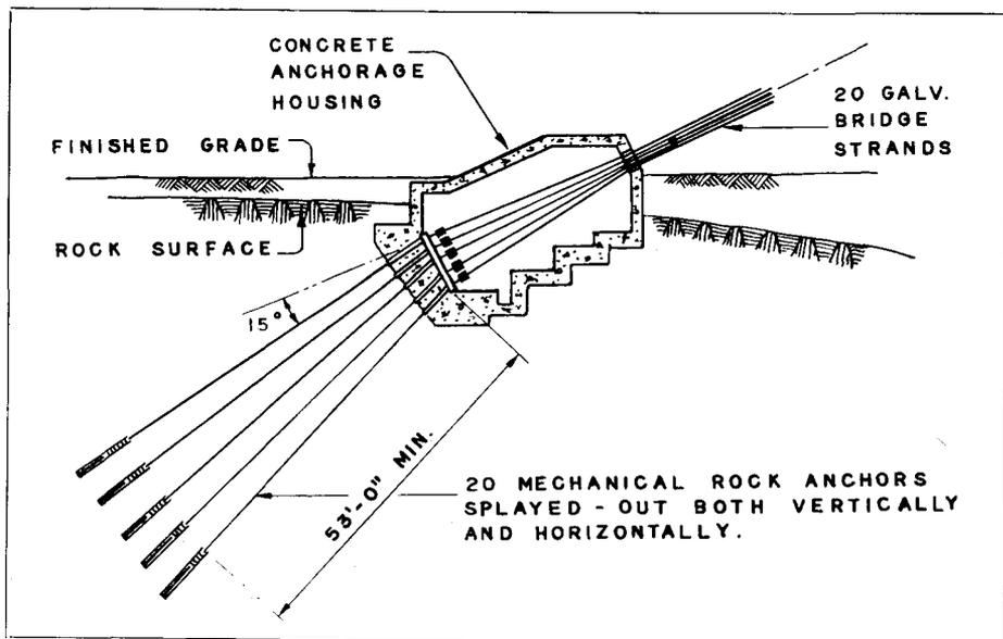
Fig. 11—Anchorage Housing—Typical Section
