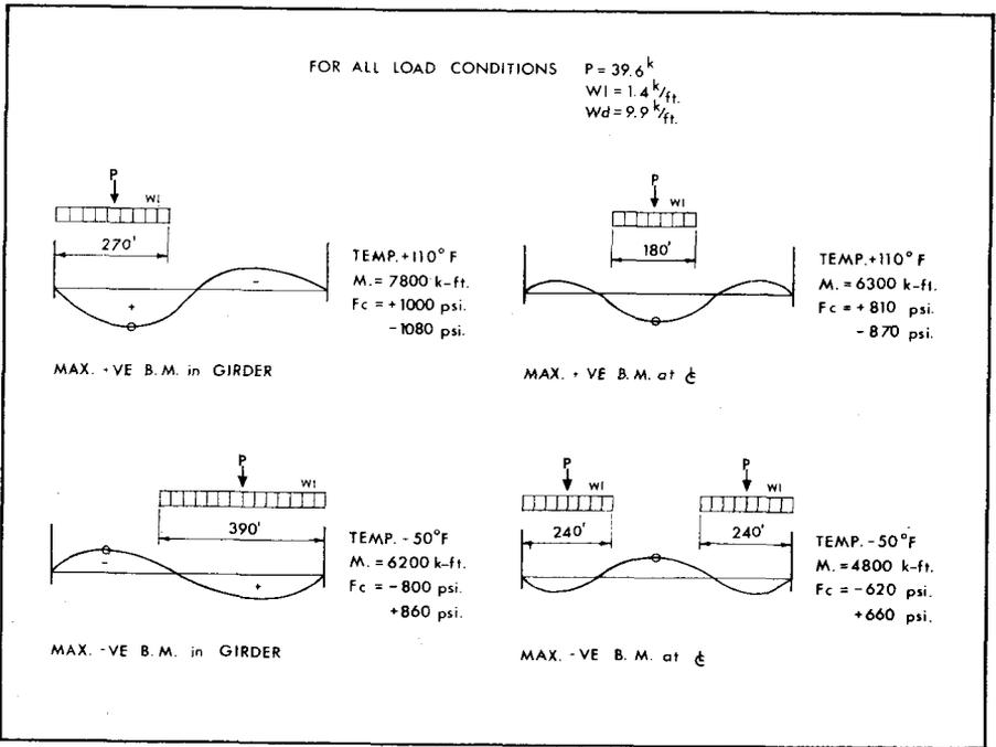
Fig. 5—Live Load Positions for Maximum Moments
