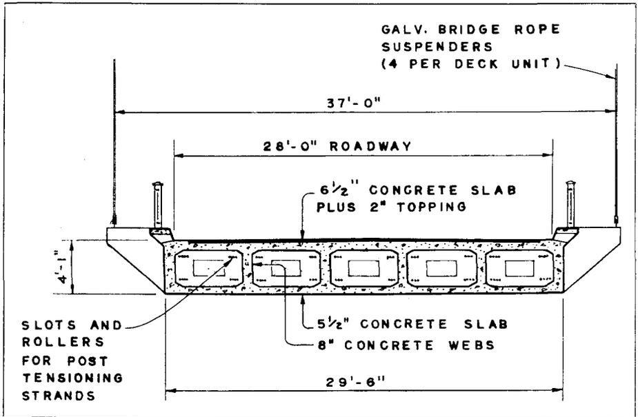
Fig. 3—Typical Section—Suspended Precast Deck Unit
