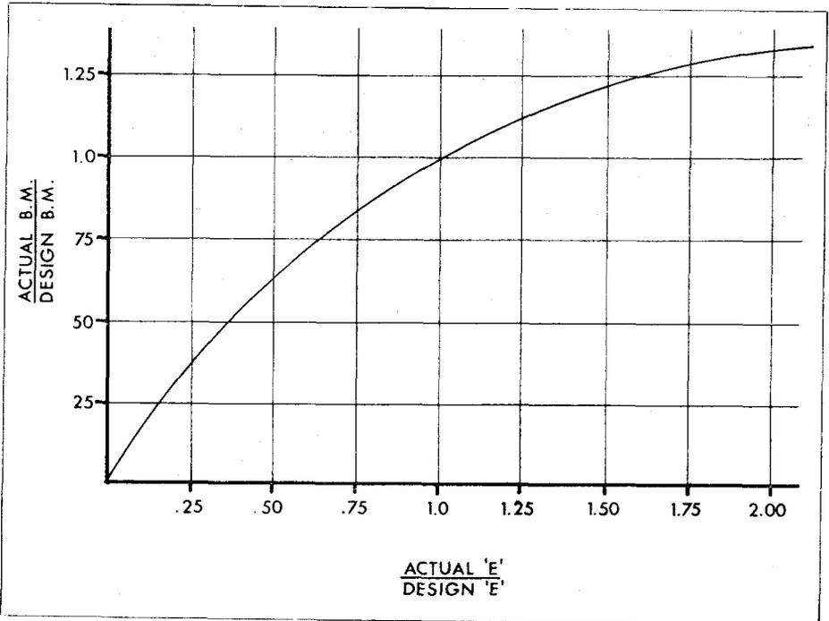
Fig. 6—Relationship between Girder Modulus and Bending Moment
