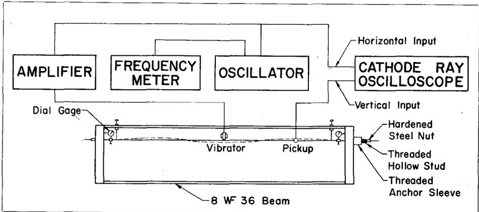
Fig. A.2—Schematic View of Test Setup.
