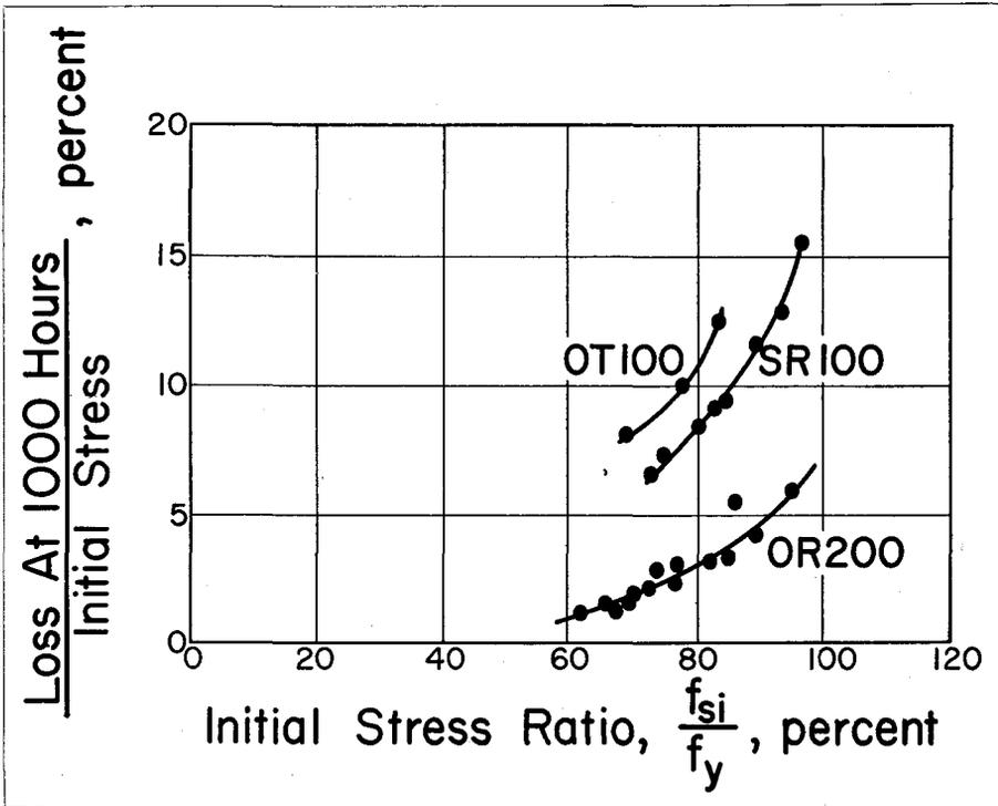
Fig. 4—Effect of Initial Stress Level on Relaxation Loss; Data from Series OT100, SR100, and OR200, Appendix A.
