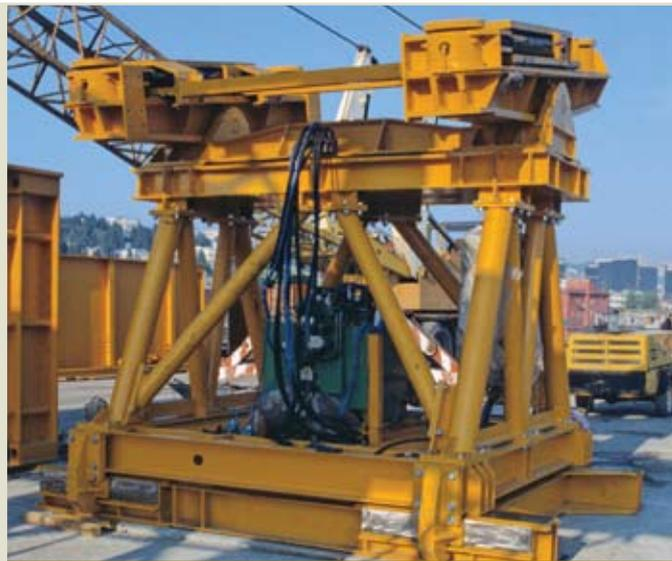
**Figure 6.** A friction launcher is assembled onto a support tower.
