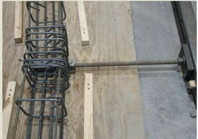
**Figure 13.** Three extra stirrups at 2 in. spacing were used at the support locations. Note: 1 in. = 25.4 mm.
