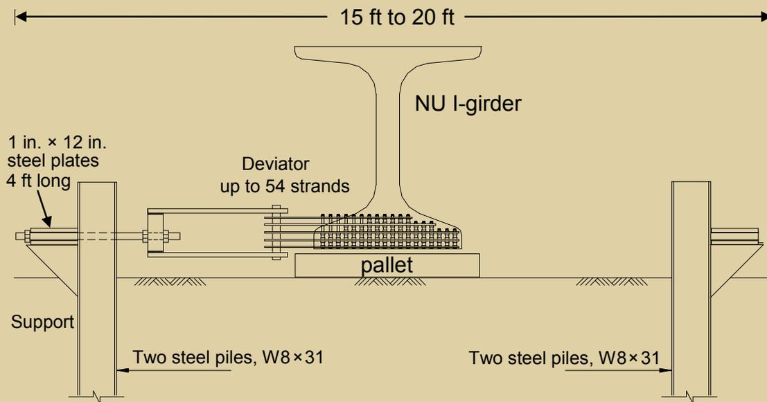
**Figure 21.** A deviator was assumed to be supported by two steel piles, cantilevered 1 ft above the ground. Note: NU = Nebraska University. W8 x 31 = 8 in. x 31 lb/ft. 1 in. = 25.4 mm; 1 ft = 0.305 m; 1 lb = 4.448 N.
