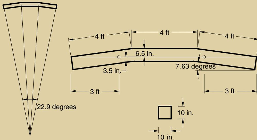
**Figure 10.** The test beam had an  $R$  of 30 ft, and steel tendons were pulled from straight lines using deviators to create chord segments with  $\theta'$  equal to 7.63 degrees. Note: 1 in. = 25.4 mm; 1 ft = 0.305 m.
