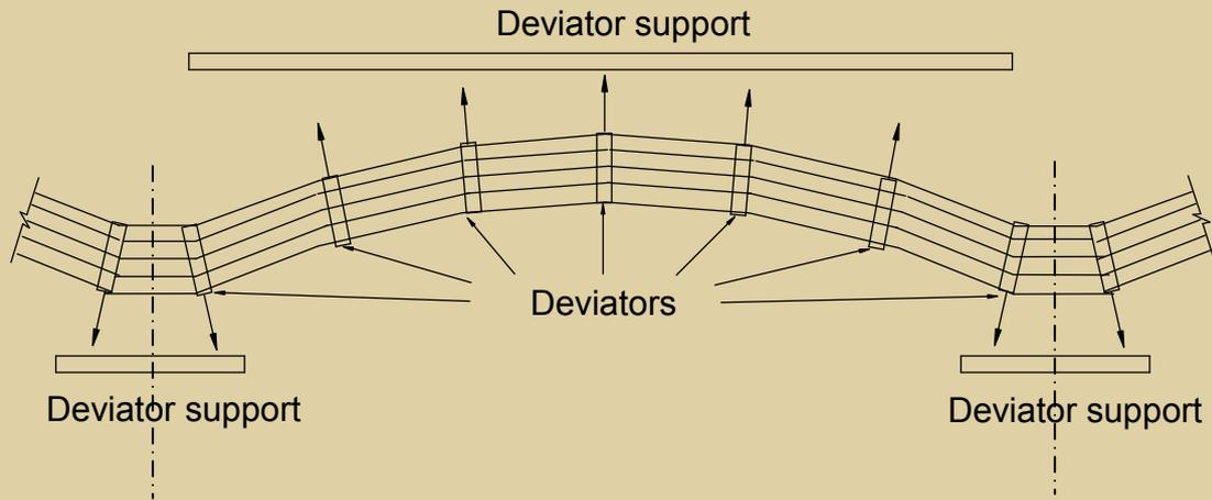
**Figure 7.** In the proposed horizontal-strand-deviation method, the deviators pull the tendons sideways at predetermined locations to create chord segments along the curve. The deviator supports must be designed to resist the pull forces from the deviators. Note: The drawing is not to scale, and the horizontal curvature is exaggerated.
