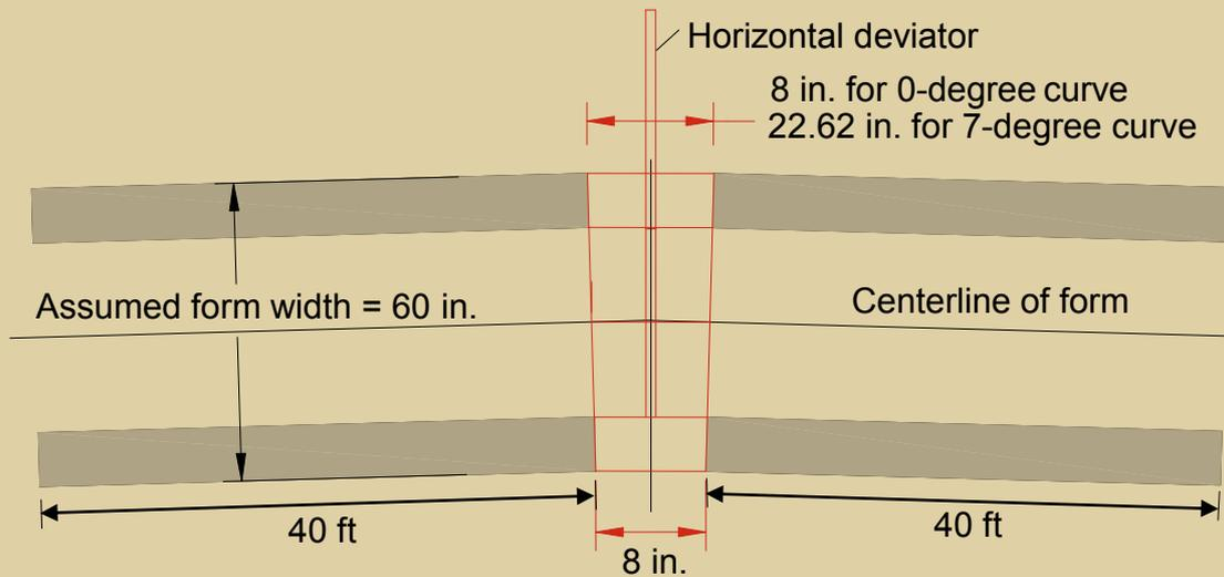
**Figure 23.** This plan view shows the joint form and deviator, which can be installed between two 40-ft-long standard forms. If an inside gap of 8 in. is assumed, then an outside gap from 8 in. to 22.62 in. would be required for 0 degrees to 7 degrees of curvature, respectively. Note: The drawing is not to scale. 1 in. = 25.4 mm; 1 ft = 0.305 m.
