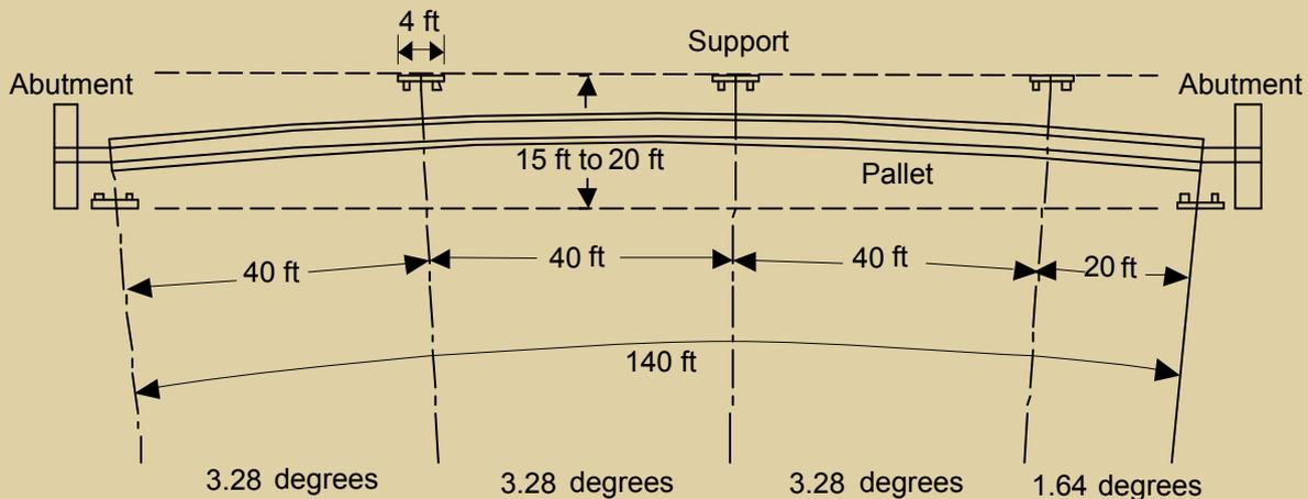
**Figure 20.** This diagram depicts the prestressing bed layout for an NU I-girder with 40-ft-long chords along a specified radius of curvature of 700 ft. Note: NU = Nebraska University, 1 ft = 0.305 m.
