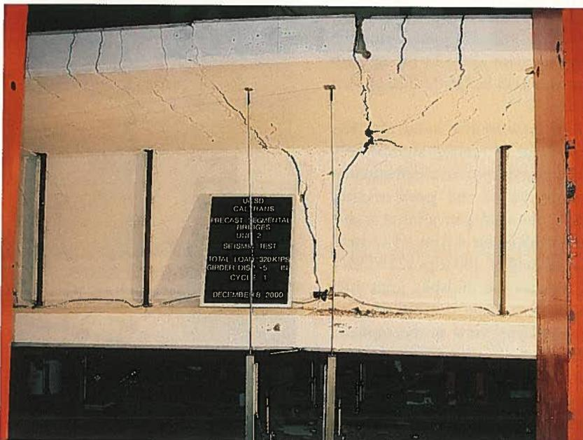
Fig. 13. Midspan joint at maximum upward displacement before failure of Test Unit 100INTCIP.
