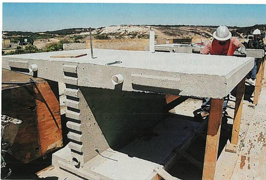
Fig. 5. A precast segment from Test Unit 100INT.
