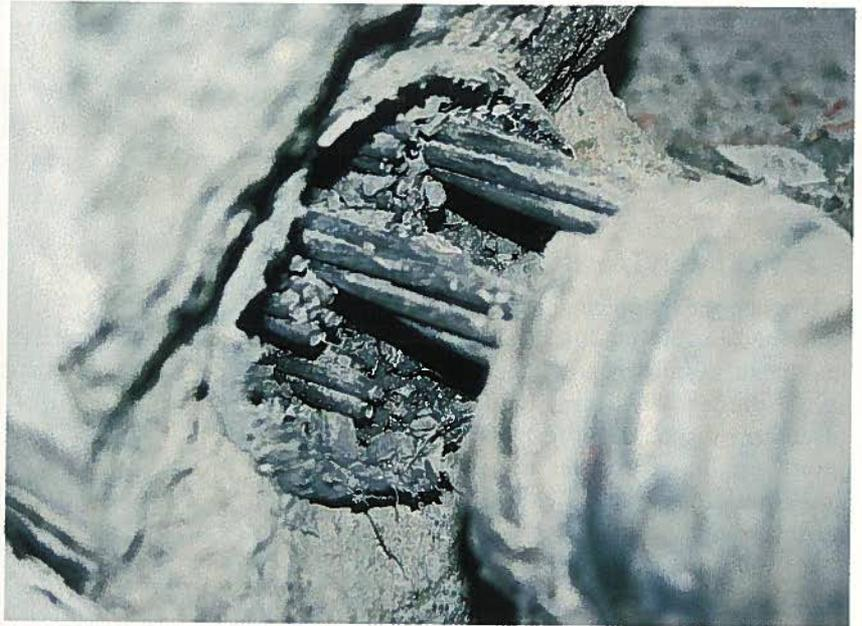
Fig. 12. Rupture of prestressing strands of Test Unit 100INT.
