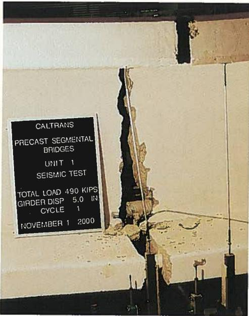
Fig. 11. Midspan joint after failure of Test Unit 100INT.
