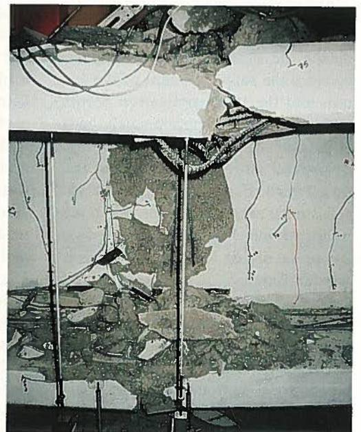
Fig. 14. Compression failure at midspan joint of Test Unit 100INTCIP.
