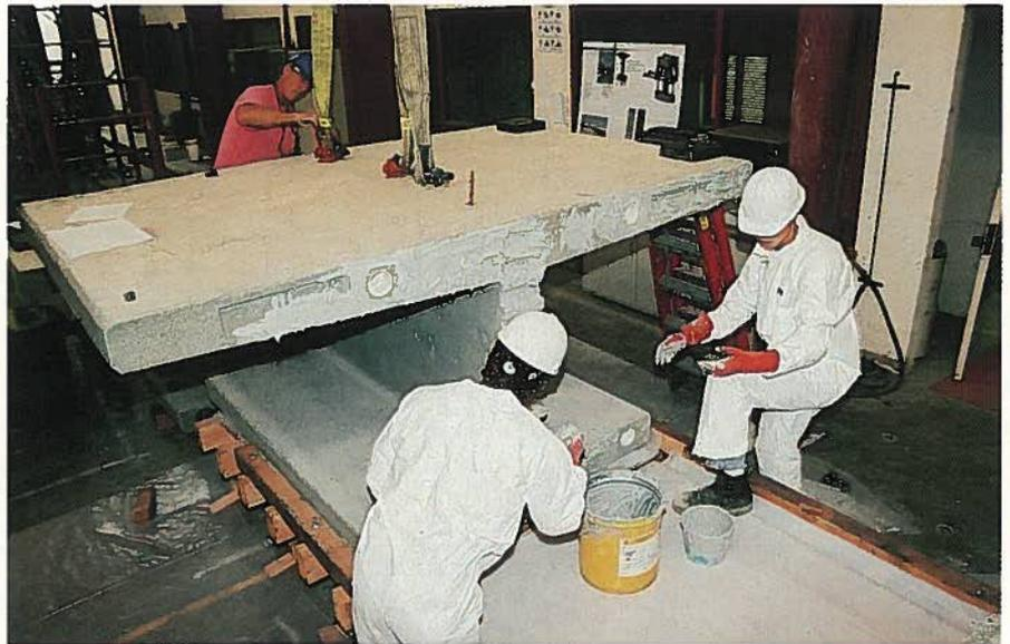
Fig. 6. Application of epoxy to the joint surface.
