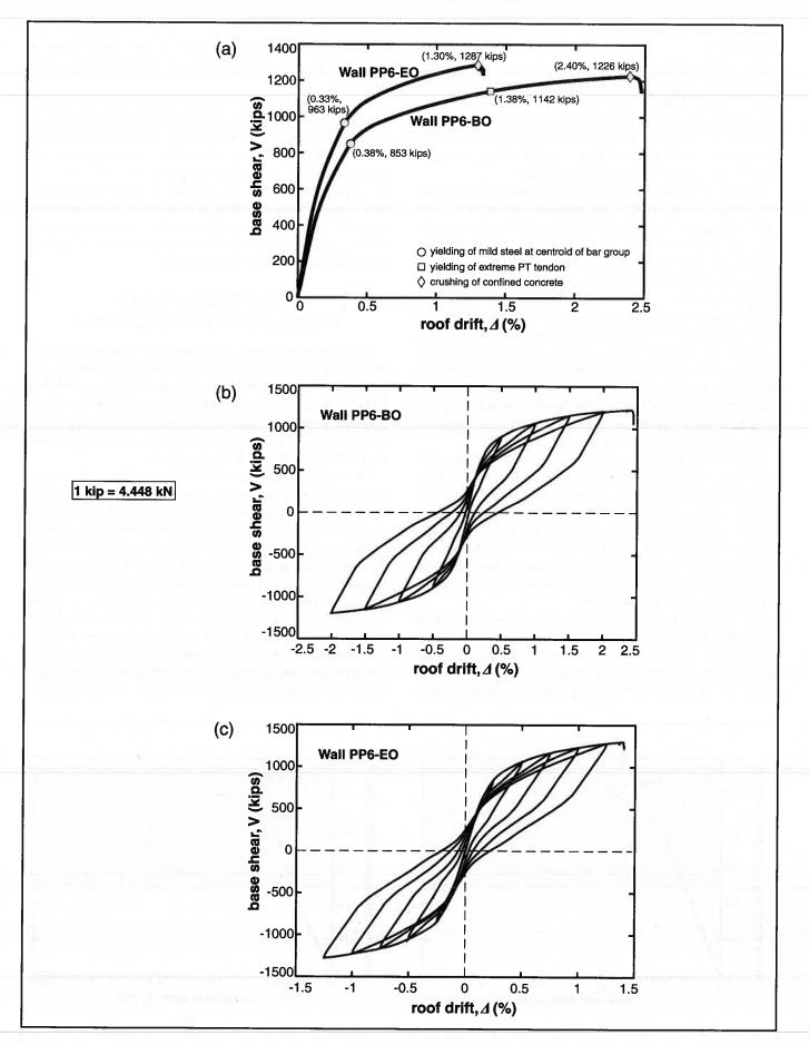
Fig. 6. Behavior of the prototype walls under lateral loading: (a) monotonic loading; (b) cyclic loading, Wall PP6-BO; (c) cyclic loading, Wall PP6-EO.
