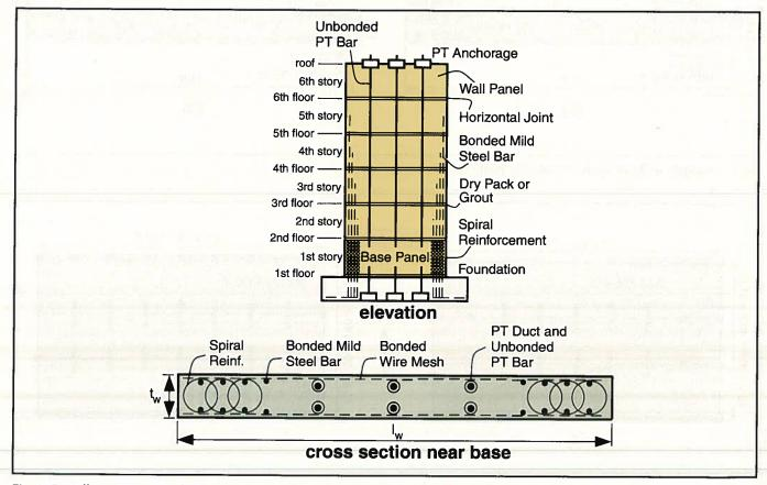
Fig. 1. Partially post-tensioned precast concrete wall.
