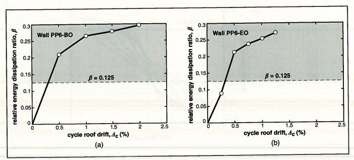
Fig. 7. Relative energy dissipation ratio,  $\beta$ : (a) Wall PP6-BO; (b) Wall PP6-EO.
