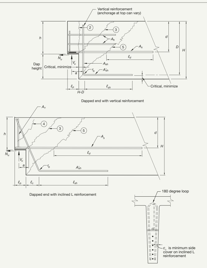
Page 5–78, Figure 5.5.5: Add the following note to figure: "Note: See Eq. 5-73, 5-74, and 5-75 for limits on the shear strength for a distance of 2H beyond the dap."
