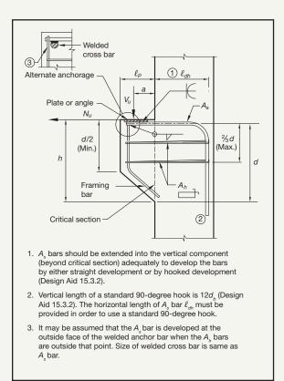
Page 5-101, Figure 5.7.2: Replace figure with the following. Change replaces h/2 dimension at the face of the corbel with d/2.
