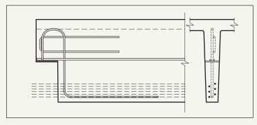
Page 5–77, Figure 5.5.4 (c): Replace figure with the following to delete the C-shaped  $A_h$  reinforcement:
