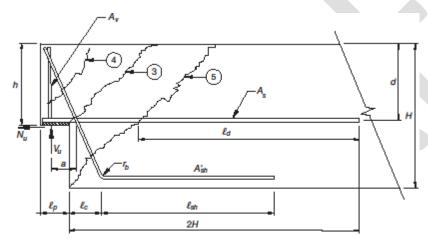
Dapped end with inclined L reinforcement
