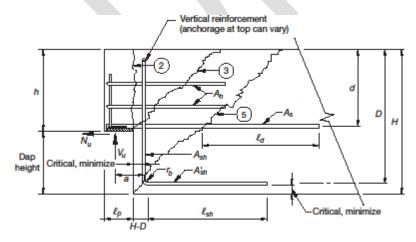
Dapped end with vertical reinforcement
