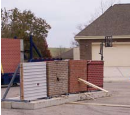
Test three smashed a 2 x 4 through a brick home with steel framing. This damage is still rather significant, but in this test the projectile did not travel through the wall. Looking at the back side shows it would take only slightly more force to push all the way through.
