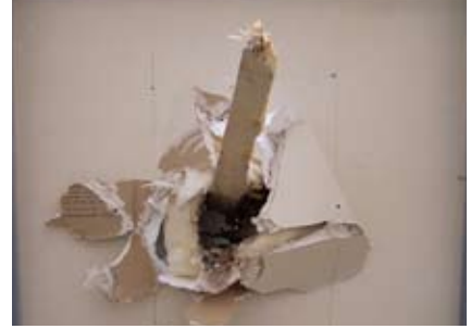
Test two shot the 2 x 4 through a brick wall with wood frame. Surprisingly, it's not all that much safer than siding. What you don't see are the pieces of brick that went flying through the back side of the panel. This wall introduced even more projectiles into the house.
