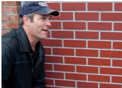
Now for the real test: hurl a 2 x 4 at a precast wall panel at 112 mph. The result: no damage visible, not even a chip.
