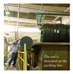
production. Pickling, which is a chemical method of descaling, is a process where the rod is given an acid bath and the chemical reaction pops the mill scale off. After the rod has been pickled it is coated in a textured carrier coating that promotes lubrication adherence during the upcoming wire drawing process.
