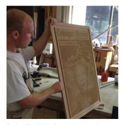
In the offset light, the image on the photoengraved master mold can be seen. A formliner will be made from this and then cast in concrete.
