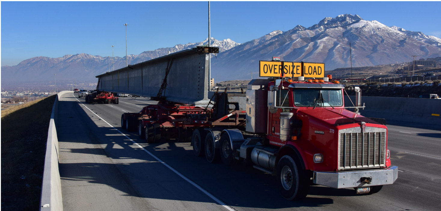
A 203 ft (61.9 m) long girder weighing 225,000 lb (102,000 kg) is shipped 27 mi (45 km) from Forterra Structural Precast in Salt Lake City, Utah, to the Interstate 15 Technology Corridor project. Courtesy of Forterra Structural Precast.
