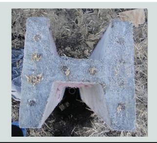
**Figure 6.1.** Ultra-high-performance concrete pile end after driving.
