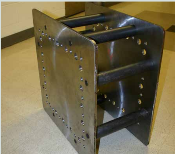
Figure A10. Splice header for 24 in. (610 mm) piles.
