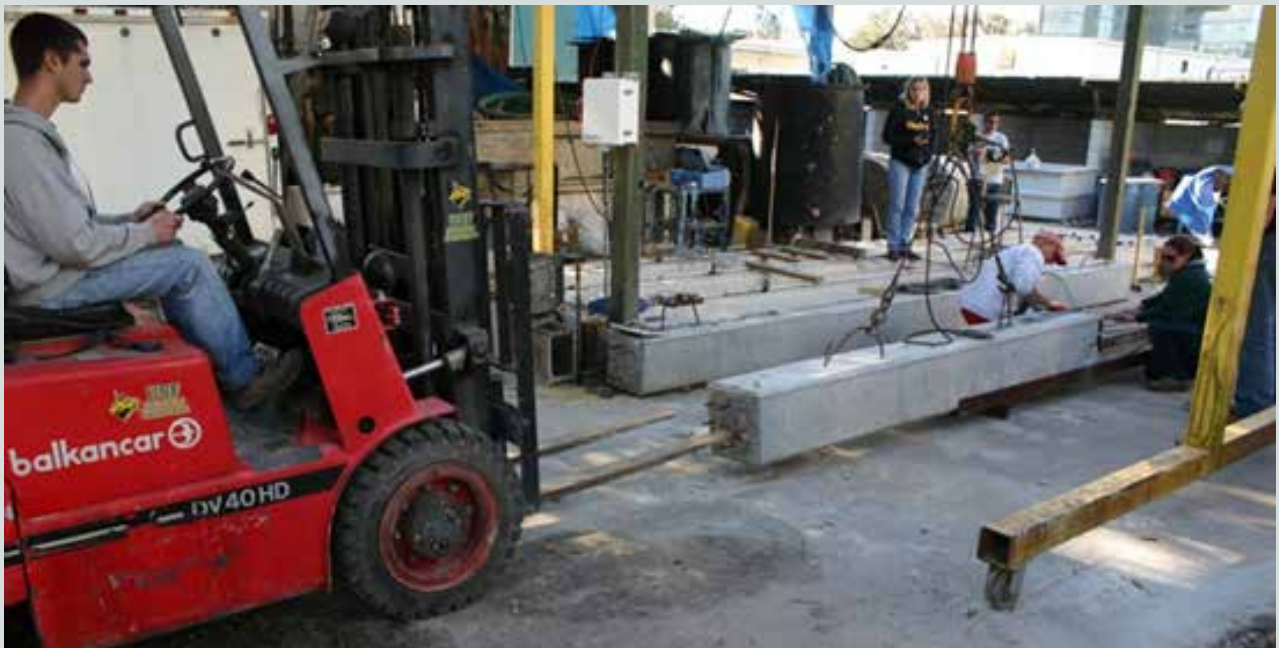
Figure A5. Weight of moving segment held by overhead crane while forklift pushed the segments together and strands were sequentially inserted into the lower segment.
