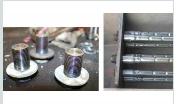
Figure A8. Deformed ducts bolted to jacking and header plates.
