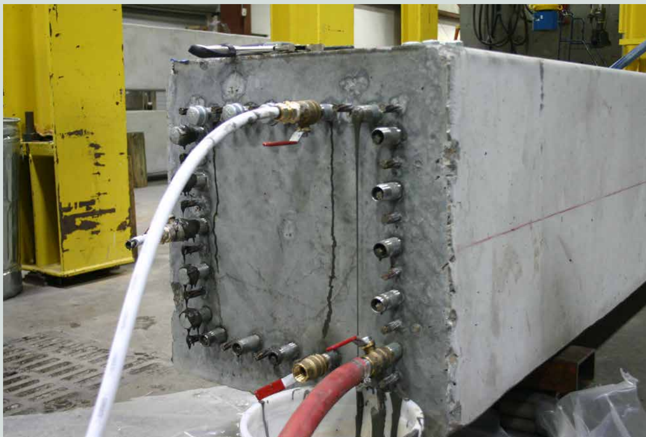
Figure A13. Grouting post-tensioned strand ducts.
