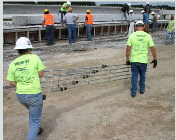
Figure A11. Five-duct interchangeable panel completed with staggered anchorages and deformed ducts.
