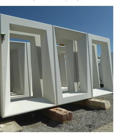
Window panels for the Domino Sugar Refinery redevelopment project in Brooklyn, N.Y., are stored at Gate Precast in Winchester, Ky. The panels were made using forms that were created with 3-D printing. Courtesy of ORNL.
