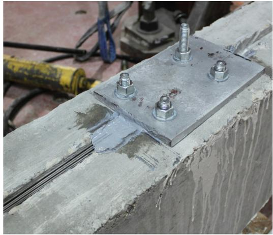
**Figure A8.** The end anchors connected to the beam.
