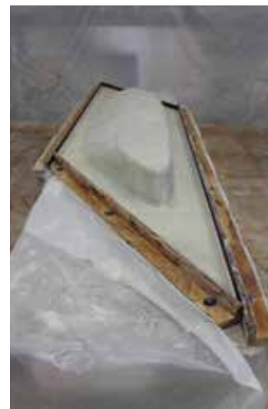
Forms for the glass-fiber-reinforced concrete panels were fabricated by precisely cutting styrofoam blocks into the desired shapes, resulting in these shapes.
