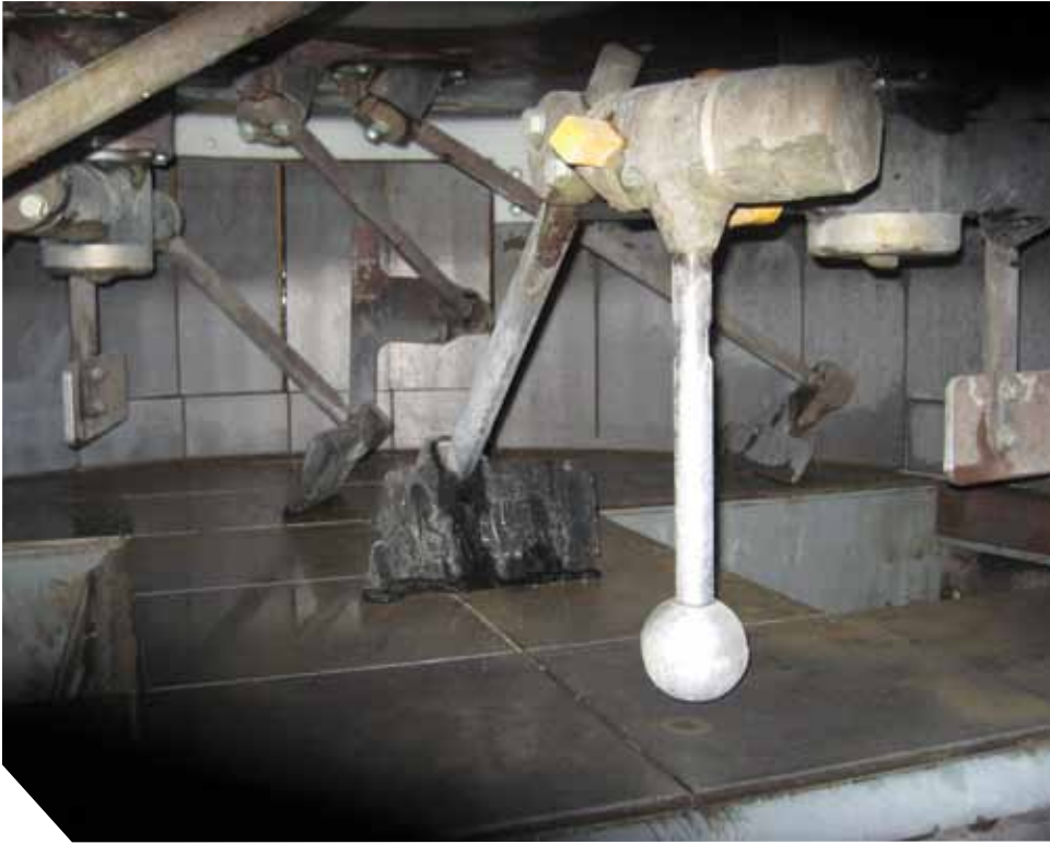
The Visco Probe, which was recently released in the United States, is designed to control the viscosity of self-consolidating concrete. Courtesy of Skako Inc.
