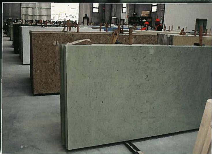
Agglonord SRL in Caprino uses no cement or water to create colorful slabs.
