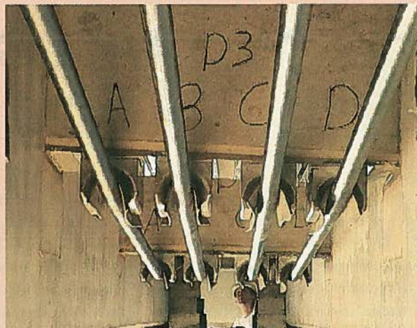
Underside view of test girder showing externally draped carbon fiber reinforced polymer (CFRP) tendons.
