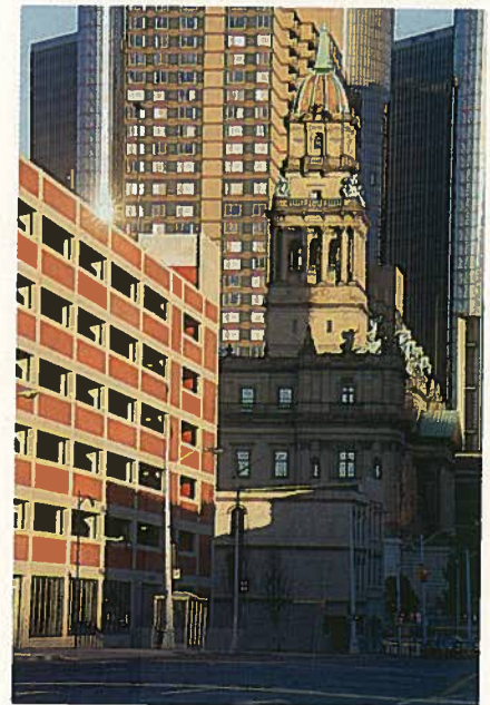
Architectural precast concrete panels with simulated brick help the structure blend with its vintage surroundings.
