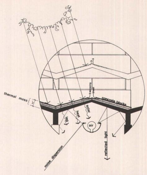
12-hour heat lag—The mass of the precast concrete roof structure provides a time lag in heat loss and heat gain. Thus, the heat gain of a summer day is delayed to act on the inside during the evening. Similarly, the cold winter night is delayed into the first shift when the production process provides excess heat.
