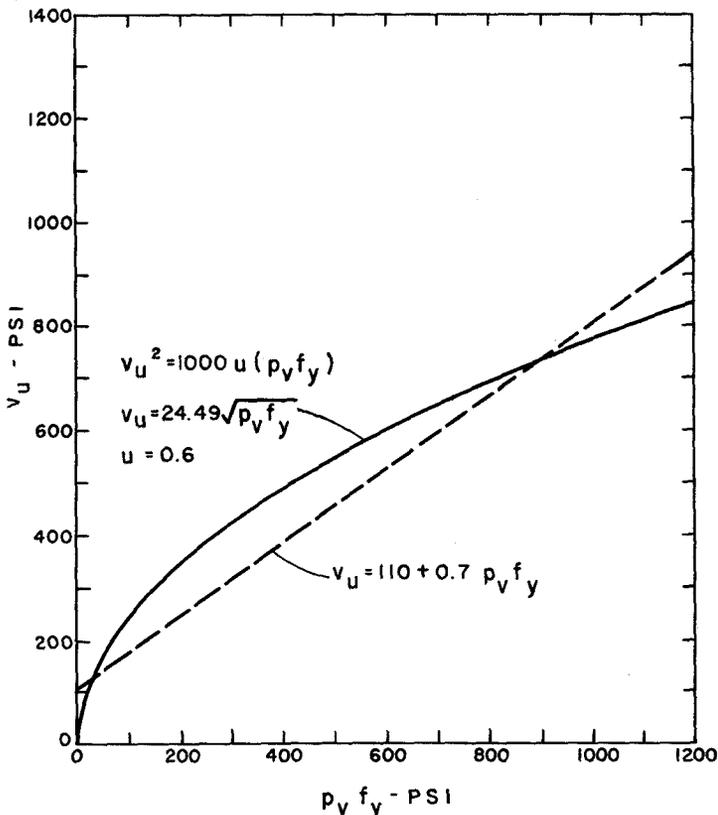
**Fig. G.  $v_u$  capacity (Reference 9) smooth interface normal weight concrete—dowel action prevented.**
