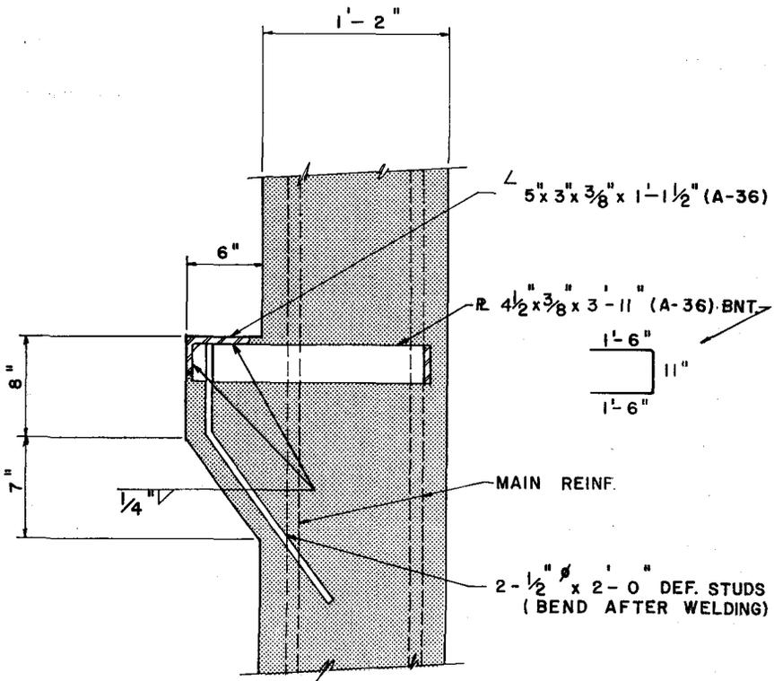
Fig. H. Modified detail using A36 steel.
