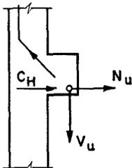
Fig. C. Force applied at bottom of corbel.
