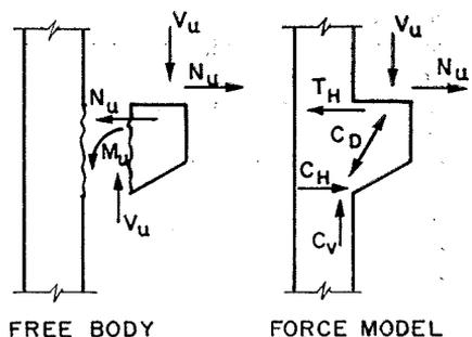
Fig. A. Typical column-corbel free body diagram and force model.
