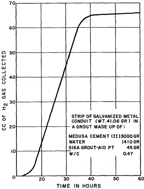
Fig. A. Gas evolved from the reaction of galvanized steel and a cement grout.
