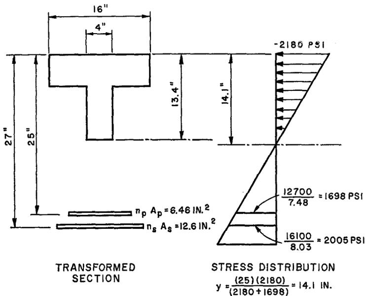
Fig. A. Stress distribution across cracked section.
