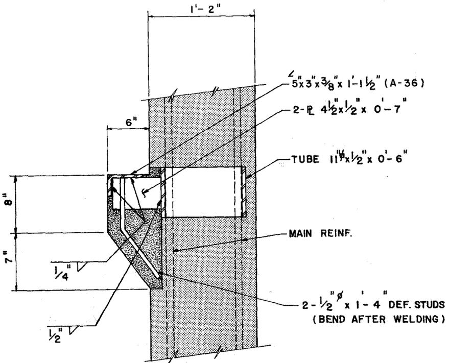
Fig. J. Modified detail using A36 steel with corbel attached after fabrication.
