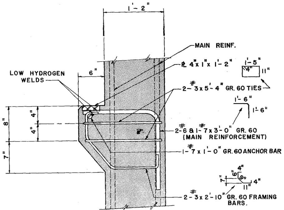
Fig. I. Author's detail using reinforcing steel cage.
