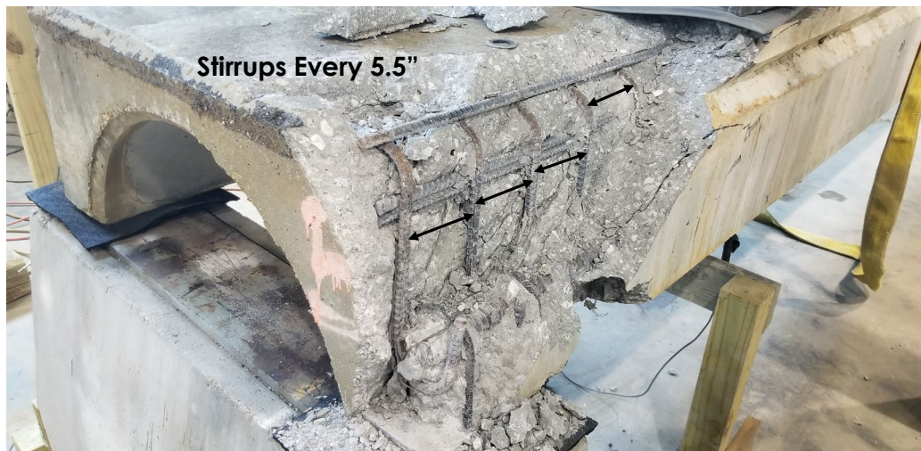
Figure 23 – Autopsy Showing Reinforcement Pattern and Bearing Plate
