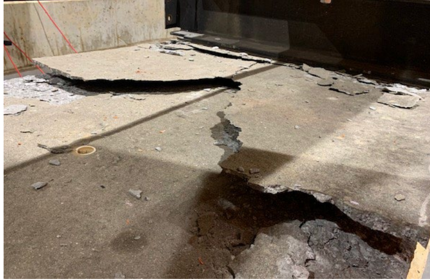
Figure 16 – Top Flange Concrete Compression Failure
