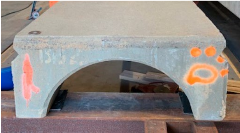
Figure 1 - Cross Section of Arch Beam
