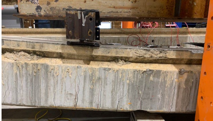
Figure 14 – Deformation at Failure
