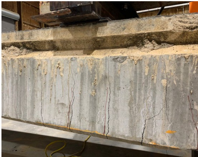
Figure 15 – Cracking near Load Point
