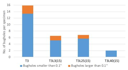
Fig. 5: Surface finish of concrete mixes with varying limestone blended cements
