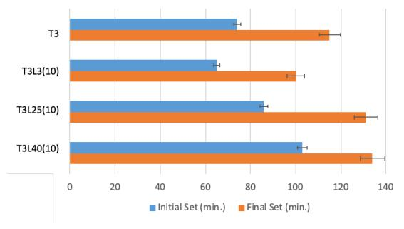
Fig. 3: Vicat time of set for Type III cement and limestone blended cements
