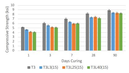
Fig. 6: Compressive strength of Type III cement and limestone blended cements
