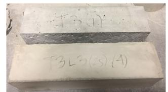
Fig. 4: Surface finish of concrete without (top) and with limestone powder (bottom)
