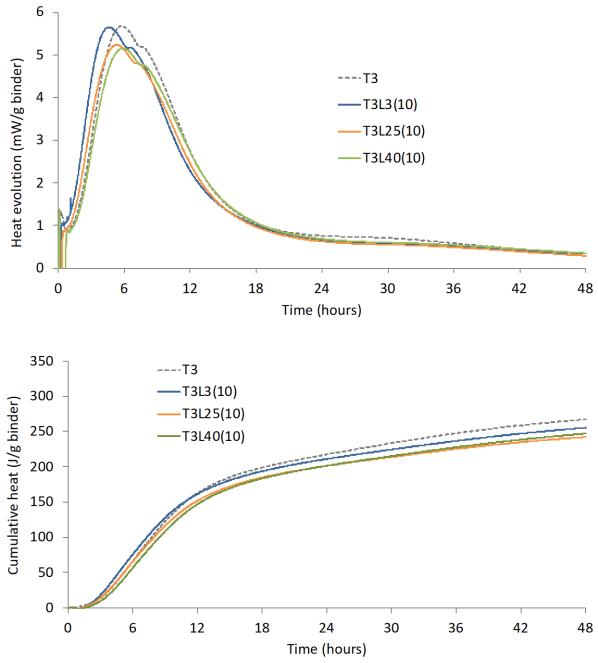
Fig. 2: Heat of hydration curve (above) and cumulative heat (below) of Type III cement and limestone blended cements
