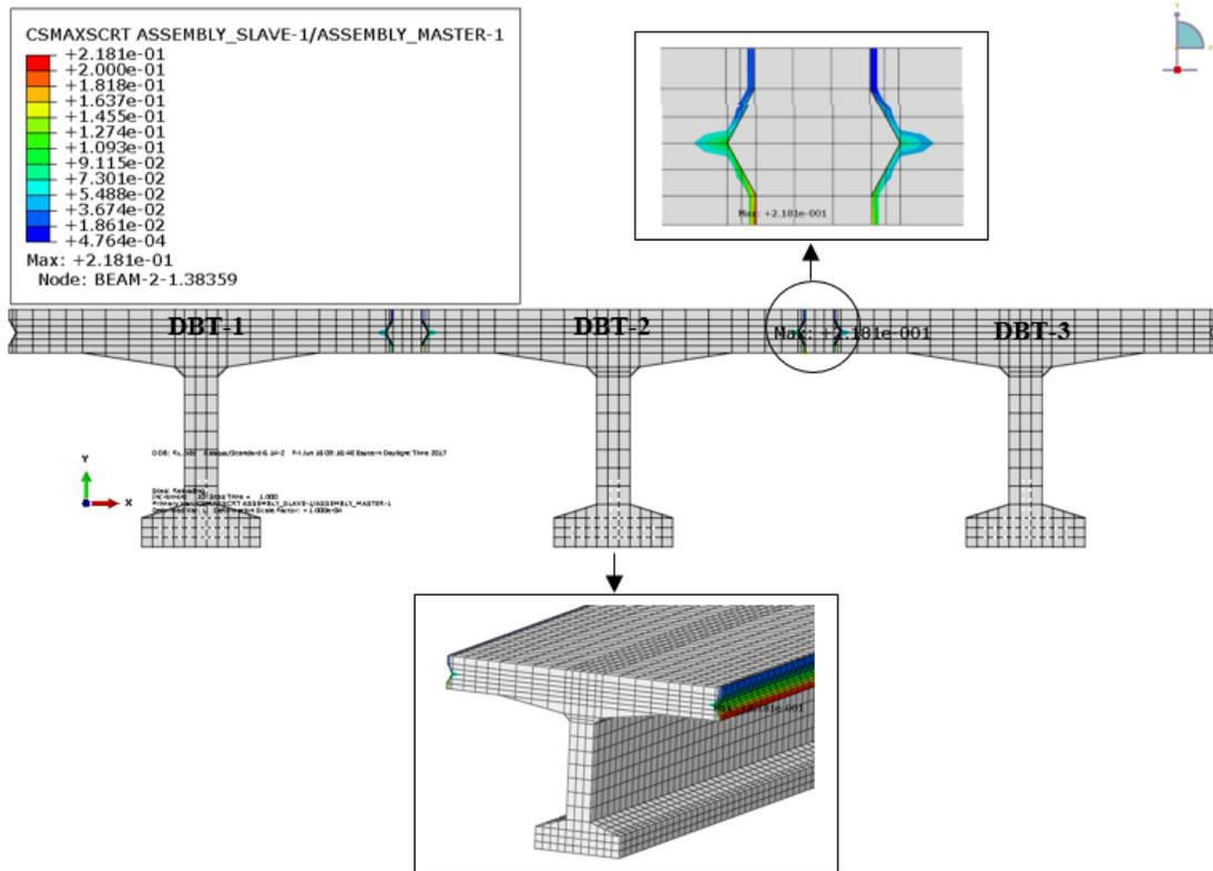
Fig. 7. Interface bond based on cohesive interaction
