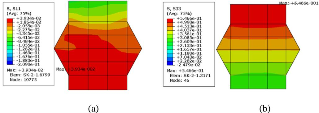
Fig. 6: Stress in shear keys under cohesive constraint: (a) transverse, (b) longitudinal
