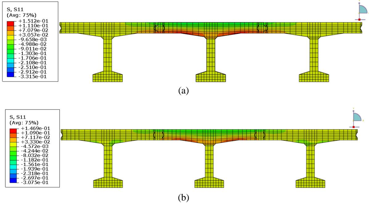
Fig. 4. Transverse behavior of DBT's at mid span: (a) tie constraint, (b) cohesive constraint
