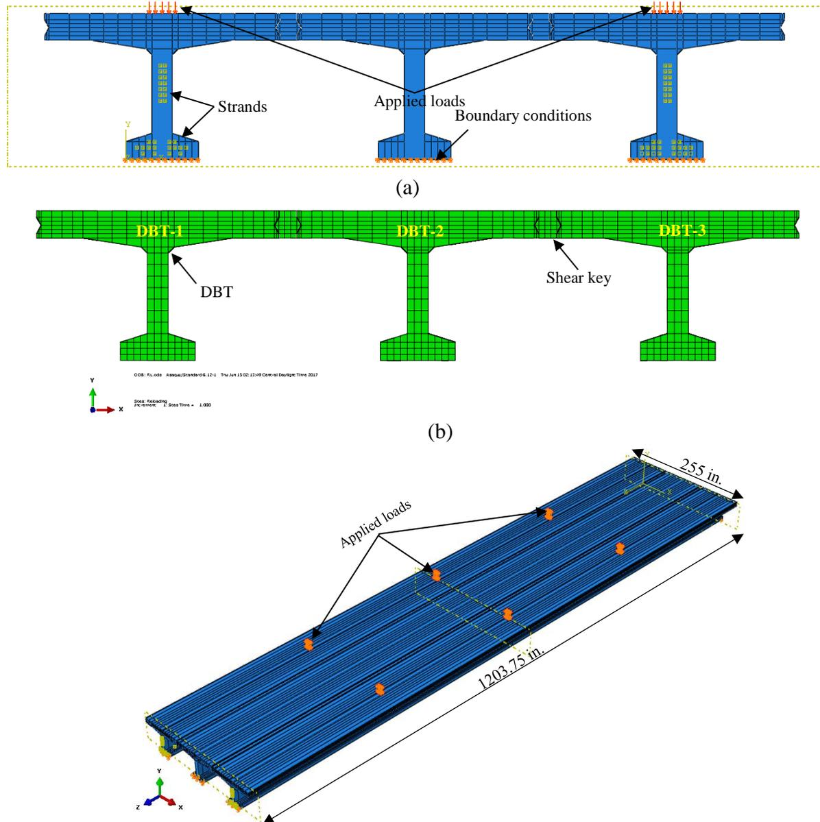
Fig. 1. Finite Element Model: (a) parts' details and boundary conditions, (b) mesh, and (c) loads
