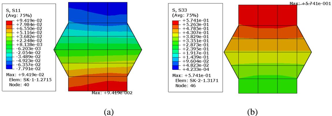
Fig. 5: Stresses in shear keys under tie constraint: (a) transverse, (b) longitudinal
