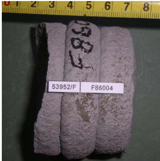
Fig. 13: Side view of sample of 3D Printed wall material. It shown that the printed layer is 20mm
