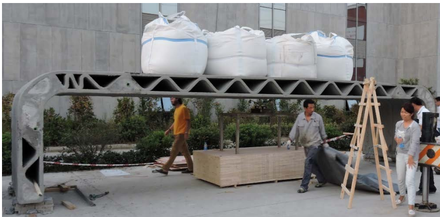
Fig. 8: 3D printed top cassette during testing
