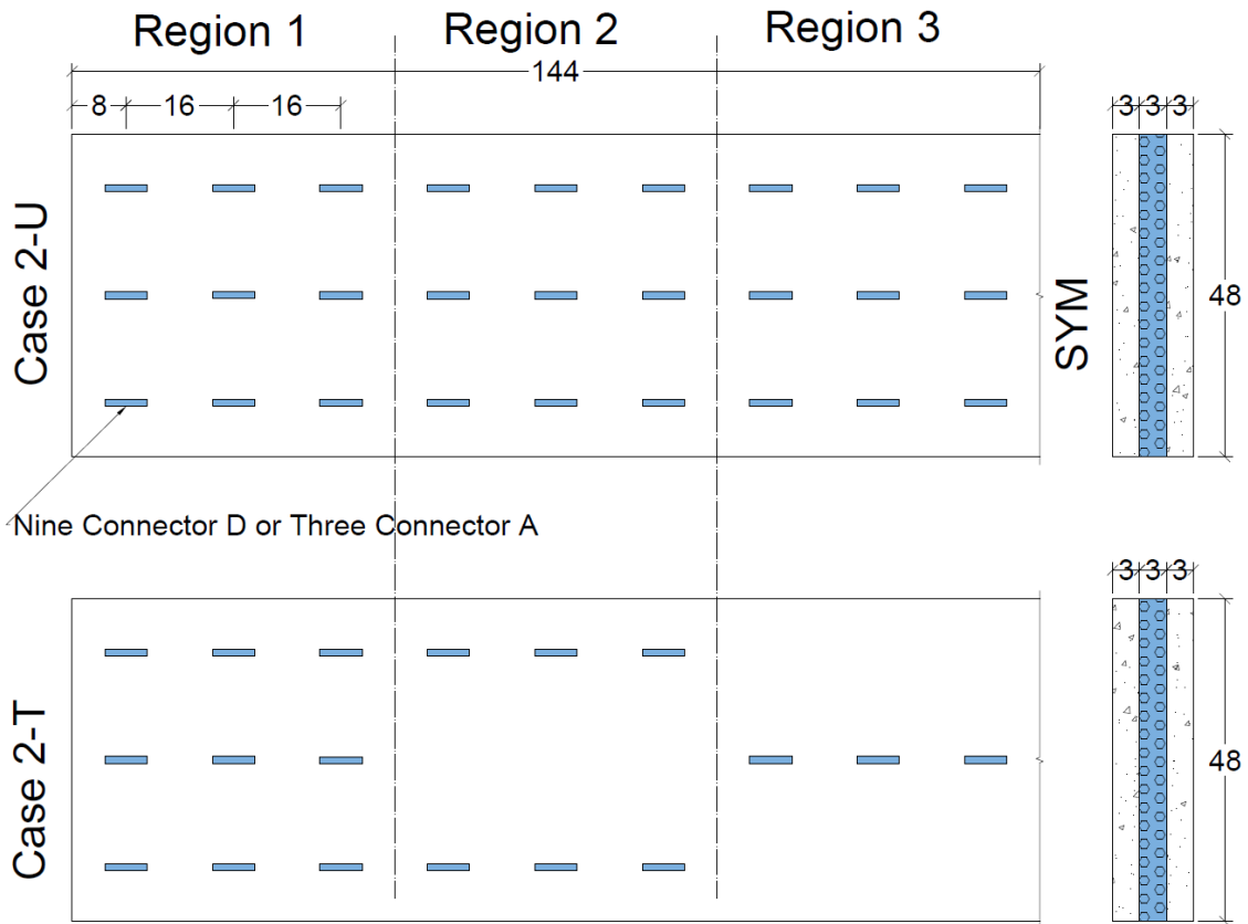
Figure 16 half symmetry of models that used parametric study in Case 2 (All units are inches)
