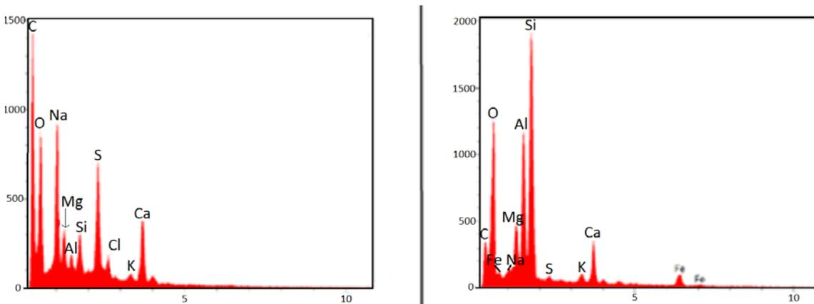
Figure 2a and 2b X-Ray Spectroscopy Results of Untreated (left) and CNS-Treated (right) Concrete
