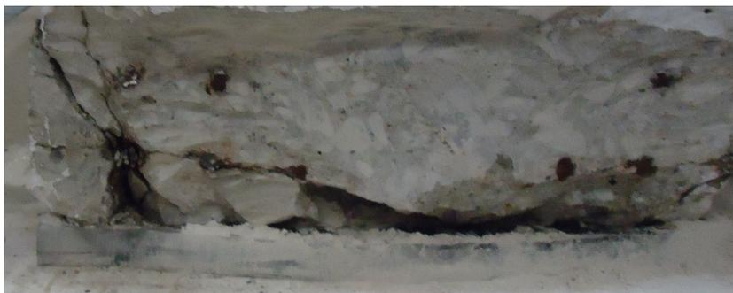
Figure 9: Spalling under load initiated by cracking caused by corrosion
