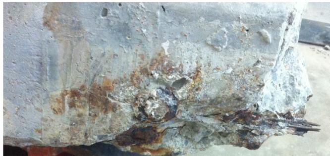
Figure 4: Corrosion at tested end for A1
