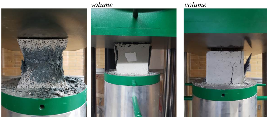
Fig. 9: Cube specimens after testing
