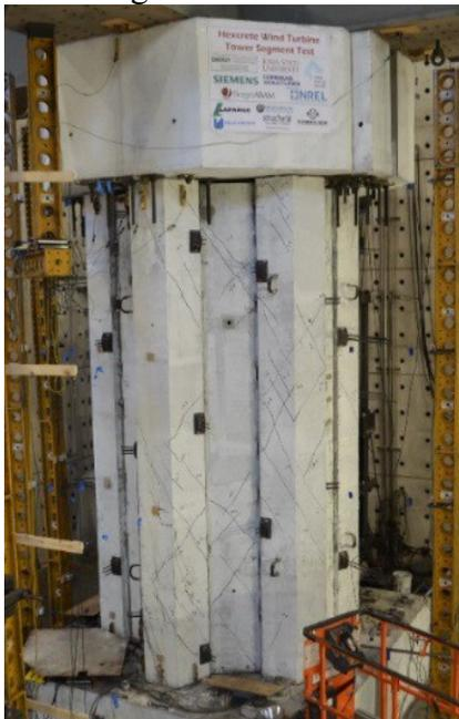
displacements demonstrated that the tower had sufficient ductility beyond extreme loads.
