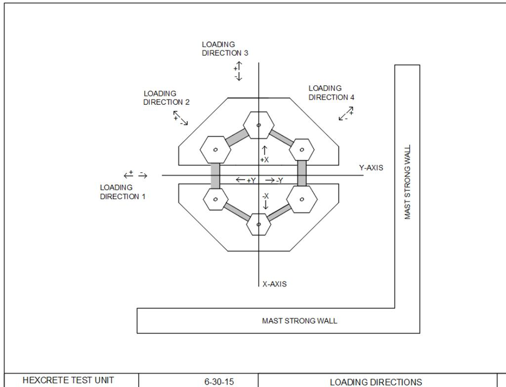
Figure 5: Test unit loading directions
