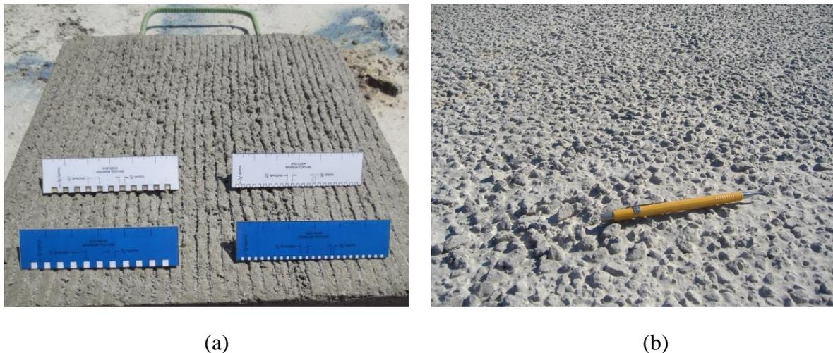
Fig. 4 Conventionally roughened (raked) surface for normal weight concrete (a) and surface of sand lightweight concrete after screeding (b).
