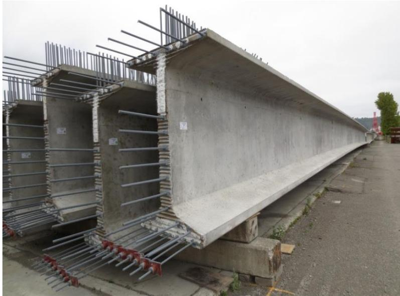
Fig. 3 WF74G Girder for SR162 Puyallup River Bridge in Storage
