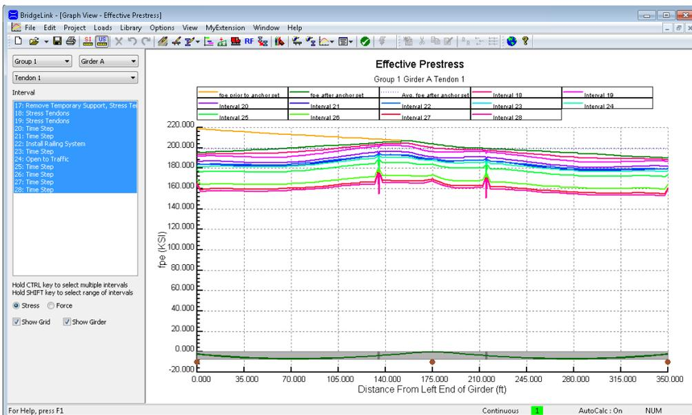
Figure 11 Effective Prestress in Tendon 1
