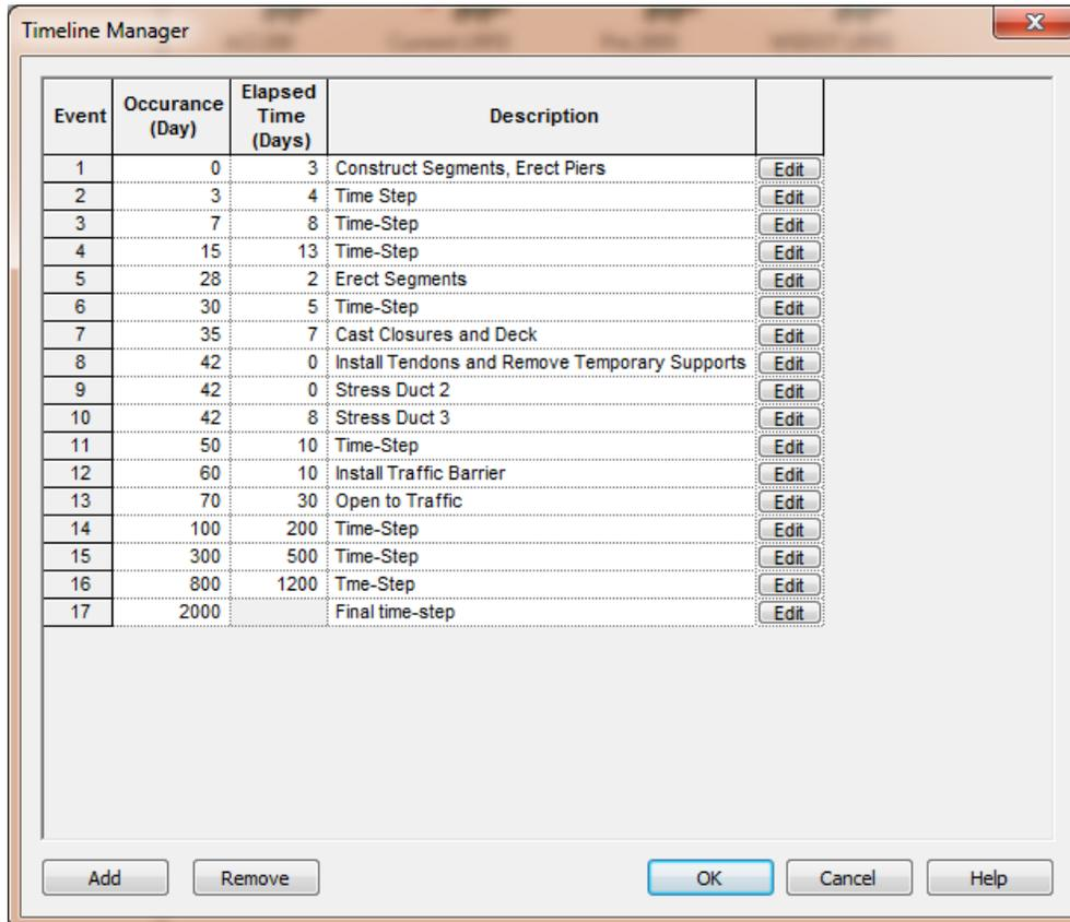
Figure 9 Construction Sequence modeled in the PGSplice Timeline Manager
