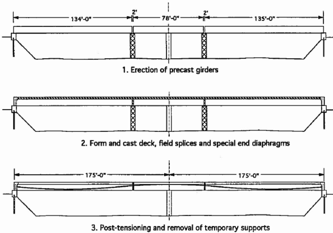
Figure 2 Construction Sequence
