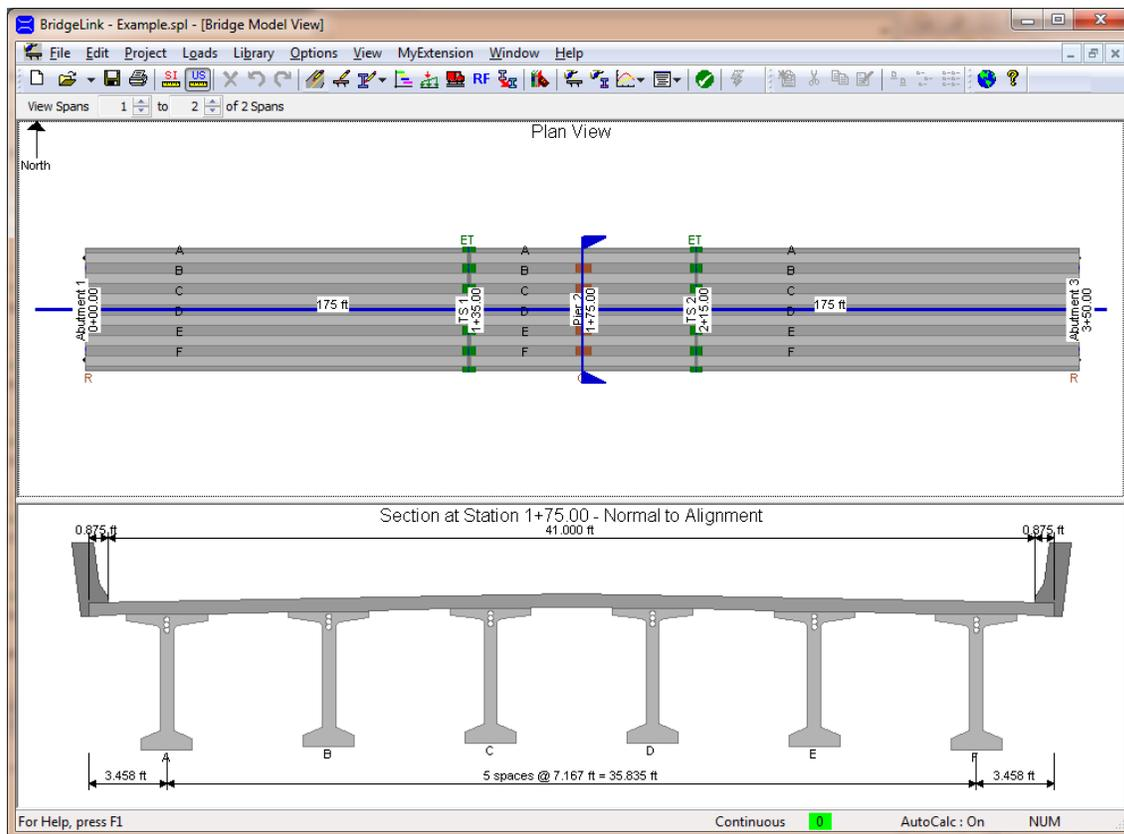
Figure 5 Model of Example Bridge
