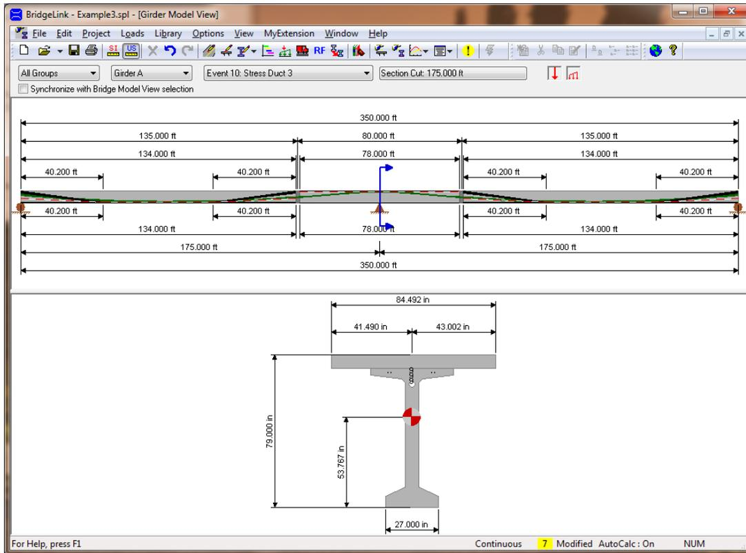
Figure 8 Section and Elevation of Spliced Girder
