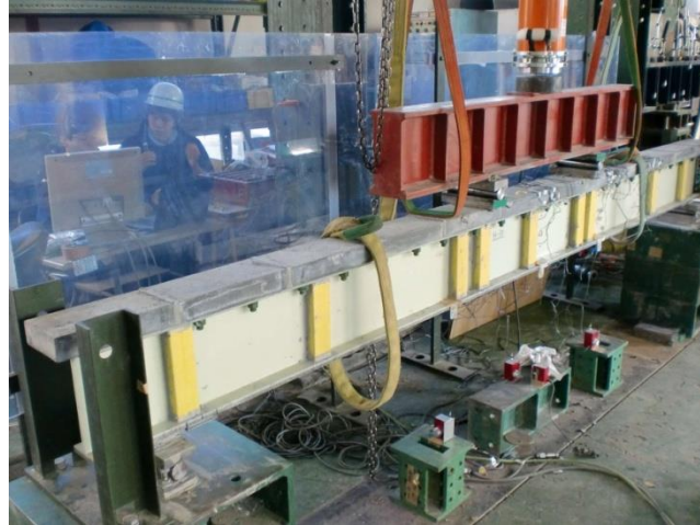
Fig. 3 Test setup of FRP-UHPFRC composite girders
