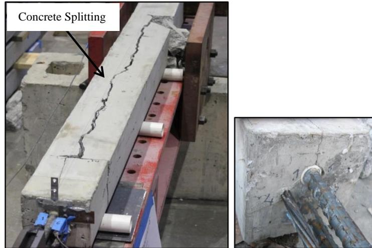
Specimen 6 (2 #No. 6 bars) after failure
