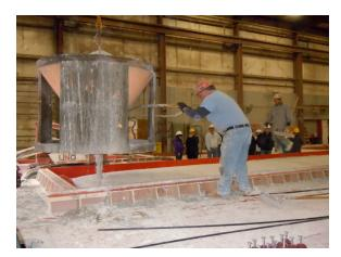
Fig. 5 Miami University architecture students observing the pouring of a precast panel
