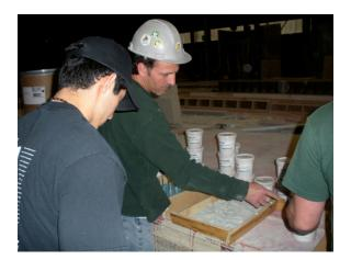
Fig. 4 Precast foreman suggesting additional reinforcement for student's formwork prior to casting.
