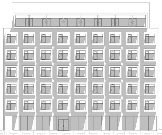
Figure 08: Simulation of shadow produced by the 12-inch horizontal solar shade. The shade was calibrated to ensure the majority of summer light and heat is kept from entering the units, while allowing ample day-lighting in the winter. Such an understanding combined with the choice of precast concrete contributed to the building's sustainability.
