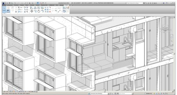
Figure 21: A cutaway section thorough the building's south façade reveals the monolithically poured front panels that contain the window boxes.
