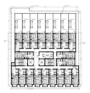
Figure 12: Second floor plan, Jersey City Micro-Housing proposal; the floors stack on levels 2-5 with additional side yard setbacks on the 6<sup>th</sup> floor.
