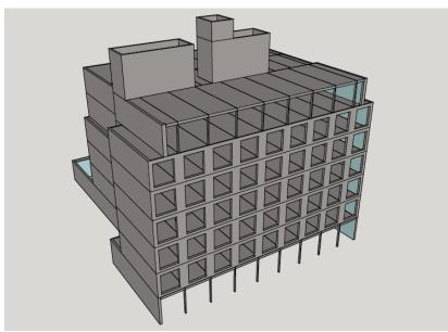
Figure 14: The selected precast company received digital data from the architect's building information model to do an initial panelization scheme for initial material take-offs and cost estimation.
