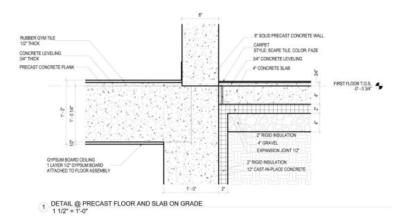
Figure 19: Precast plank to wall detail at grade. Due to the slope of the site, the building has a basement level lobby and café, which "walks out" to the sidewalk. This work is coordinated with a cast-in-place slab at the rear of the building.
