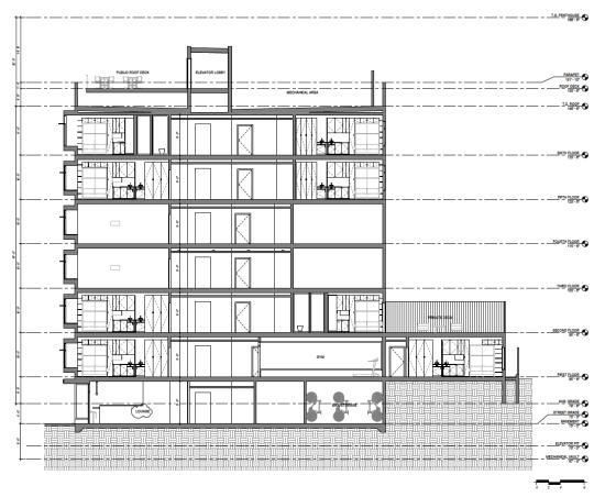
Figure 11: The existing slope of the site allowed for a basement programmed with amenity spaces including café, laundry room, and bicycle storage to be accessed directly from the sidewalk, giving the building the appearance of a 7-story building where only 6 are permitted. The first residential floor is at grade at the rear of the site, but one story up at the sidewalk.
