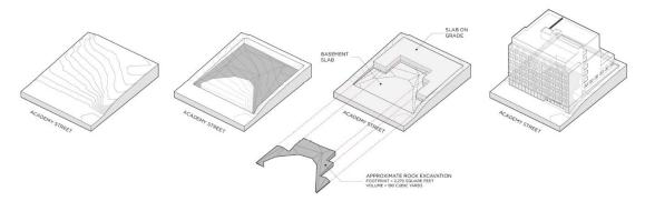
Figure 09: The sloping site in the Journal Square section of Jersey City is utilized to accommodate a basement that is accessed from sidewalk grade. The basement's perimeter is coordinated with the occurrence of rock just below grade at different locations of the site.
