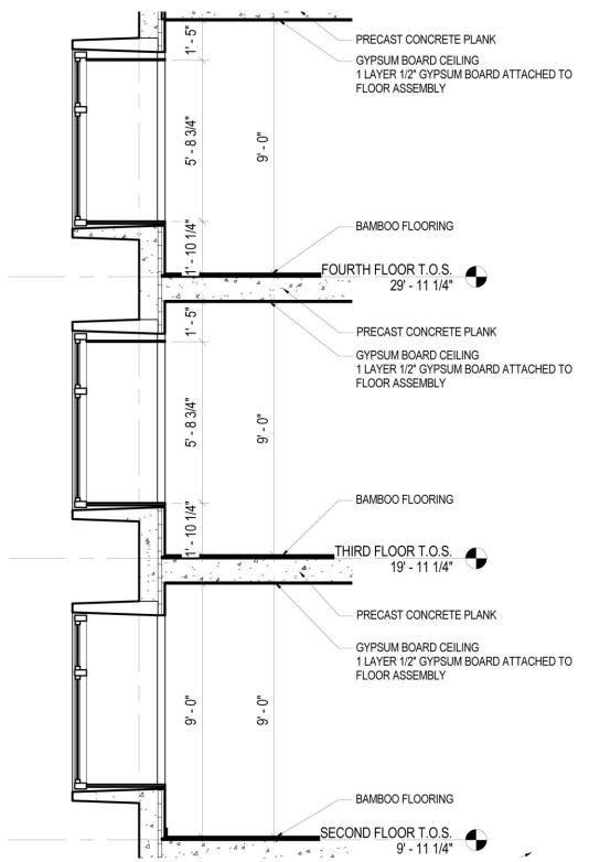
Figure 20: Shell walls use a studded precast cavity wall that connects to precast floor planks via welded steel plates. The cavity wall allows for additional insulation, which ultimately increases the energy performance of the building.
