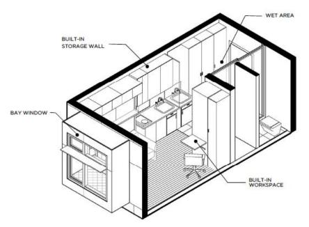
Figure 07: Cut-away of the 200 square foot unit design in GRO Architects' Micro-Housing proposal for Jersey City, NJ.
