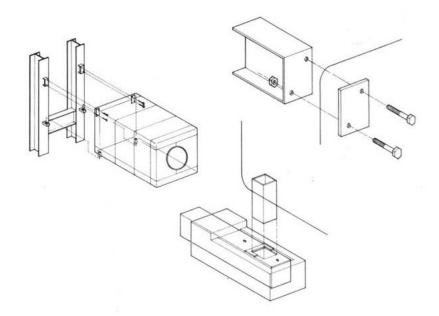
Figure 04: Units that make up the exterior of the Nakagin Capsule Tower were bolted to a steel frame with only four (4) tension bolts making it feasible to remove units for servicing.
