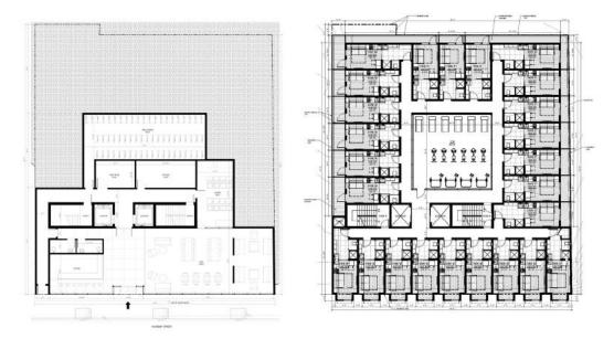
Figure 10: Basement and Ground Floor Plan, Jersey City Micro-Housing proposal, note the ground floor is actually up a story due to the slope in the site.
