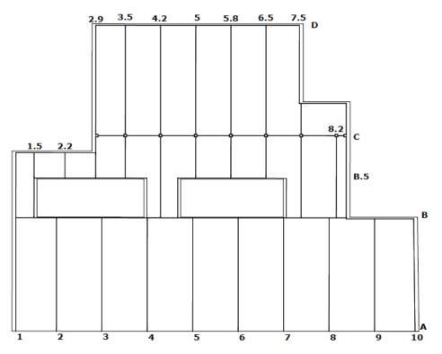
Figure 18: At the time of writing, a preliminary floor and wall plank layout had been arrived at and input into the architect's Building Information Model. The three-dimensional data would ultimately be extracted to produce the two-dimensional fabrication drawings to ultimately form the panels.
