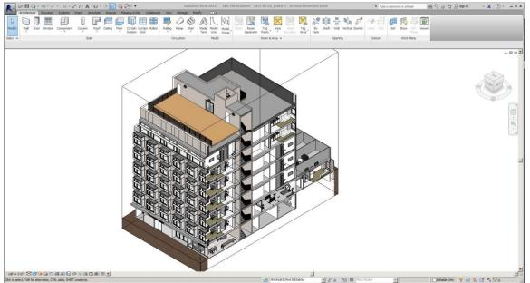
Figure 13: The architects used BIM package Autodesk Revit® to complete schematic design and move into the construction documentation phase of the project.
