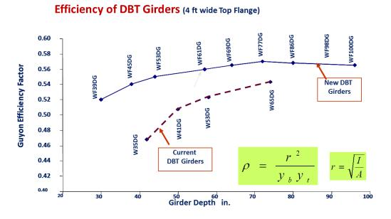
Figure 3: Efficiency of wide flange deck girder
