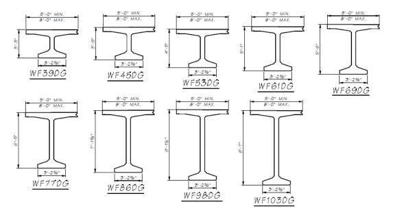
Figure 2. WSDOT Pretensioned Wide Flange Deck Girders.
