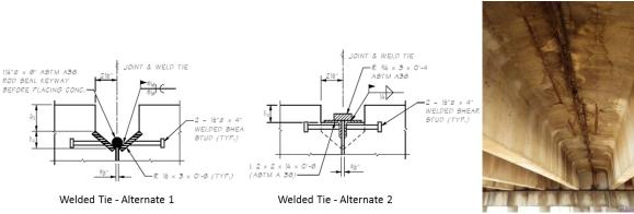
Figure 4: Connection of Deck Beam Elements
