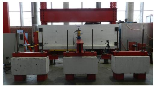
Figure 3: Test at Mid-span (Inner Failure)
