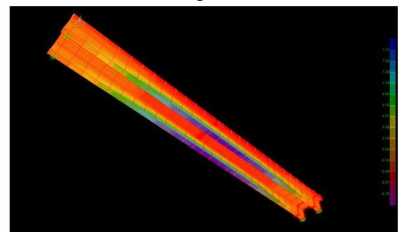
Fig. 5 Stress contour under HL-93 loading
