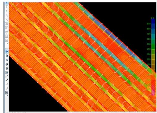
Fig. 10 Stress contour of  $S_{11}$  in bridge beams under combined loadings for Case 1-1
