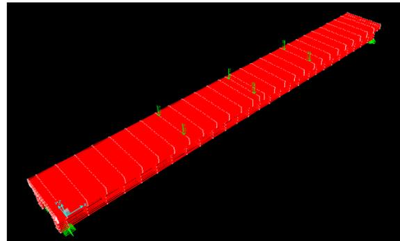
Fig. 3 Truck load HS-20 with Dynamic impact
