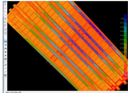
Fig. 14 Stress contour of  $S_{11}$  in bridge beams under combined loadings for case 2-1
