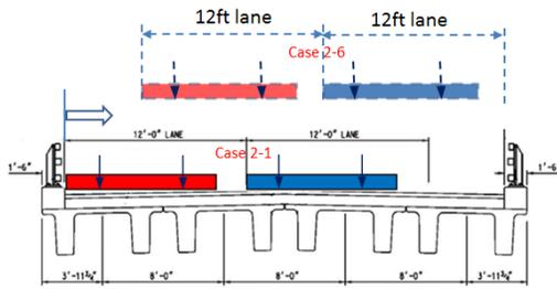
Fig 11 Loading profile for Case 2-1 (note: bridge section adapted from [2])
