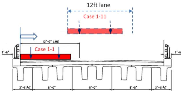
Fig. 7 Loading profile for Case 1-1 (note: bridge section adapted from [2])
