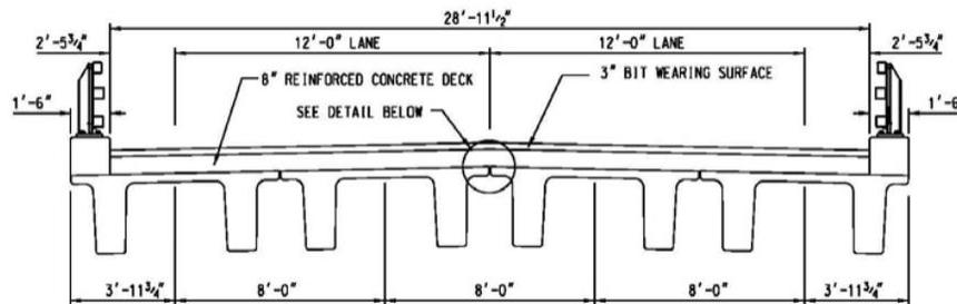
Fig. 6 Bridge section with minimum width beams<sup>2,3</sup>
