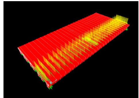
Fig. 8 Design lane load for Case 1-1
