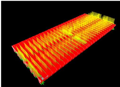
Fig. 13 Design lane load for Case 2-1
