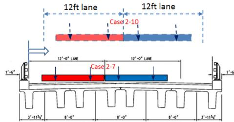
Fig. 12 Loading profile for Case 2-7 (note: bridge section adapted from [2])
