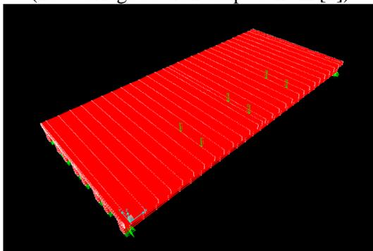
Fig. 9 HS-20 truck load with dynamic impact for Case 1-1
